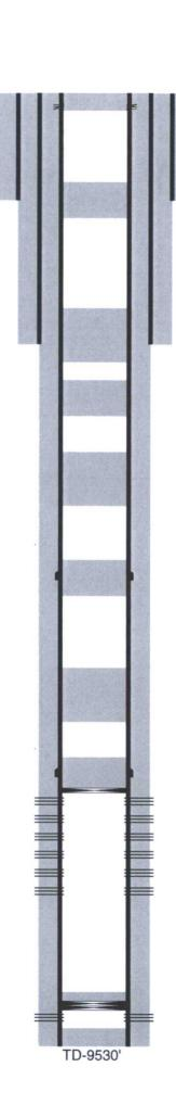
**Perf** @ **140'** 17-1/2" hole @ 1075' 13-3/8" csg @ 1075' w/ 1200sx-TOC-Surf-Circ
