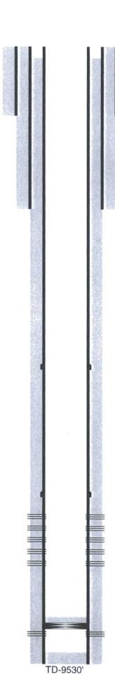
17-1/2" hole @ 1075' 13-3/8" csg @ 1075' w/ 1200sx-TOC-Surf-Circ
