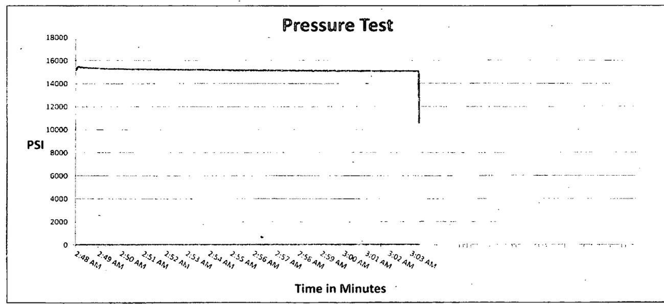
**Test Pressure** 15000 PSI      **Time Held at Test Pressure** 15 1/4 Minutes      **Actual Burst Pressure**      **Peak Pressure** 15410 PSI
