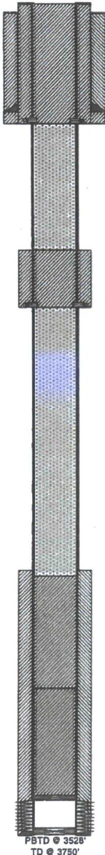
3. PUH & perf @ 405' & sqz 90 sx Class "C" cmt from 405' to surf. Attempt to CIRC 4 1/2" to surf. (Surf Shoe & Water Board)
