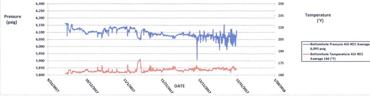
FIGURE 10: ZIA AGI #1 AND #D2 DIFFERENTIAL PRESSURE
