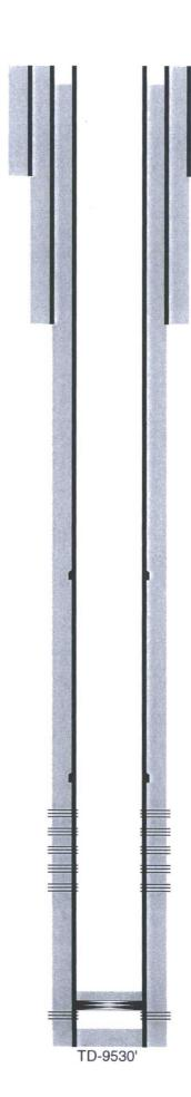
17-1/2" hole @ 1075' 13-3/8" csg @ 1075' w/ 1200sx-TOC-Surf-Circ
