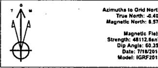
To convert a Magnetic Direction to a Grid Direction, Add 8.57°
