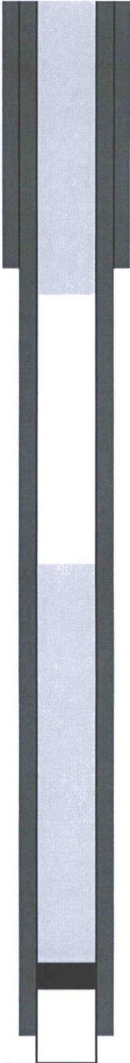
CUT OFF WELLHEAD 3' BELOW GL
