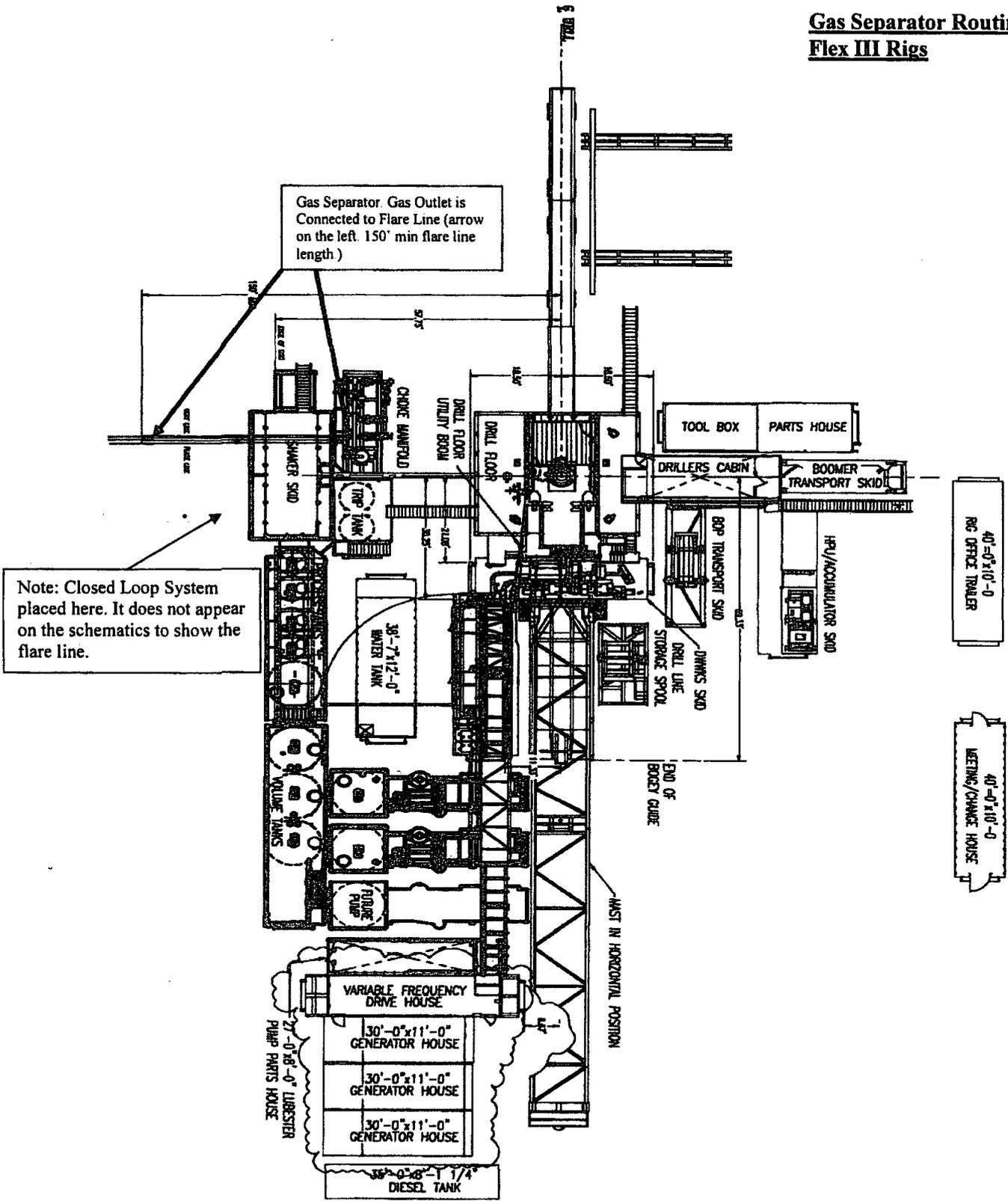
**Choke Manifold – Gas Separator (Top View)**
