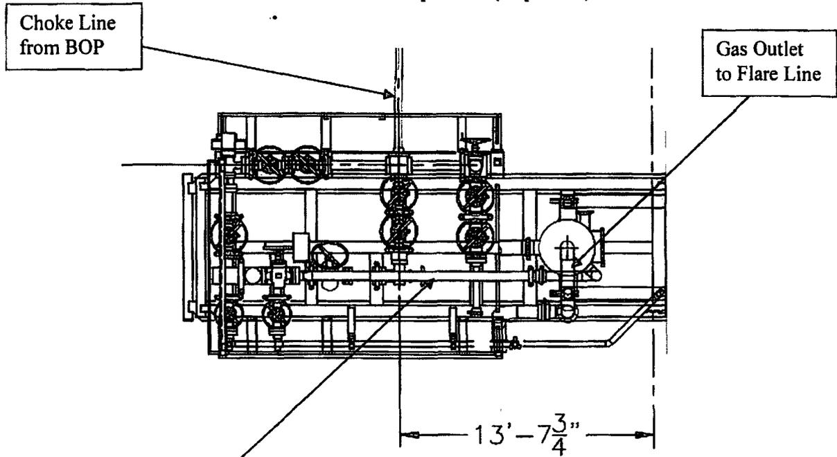
**Choke Manifold – Gas Separator (Side View)**
