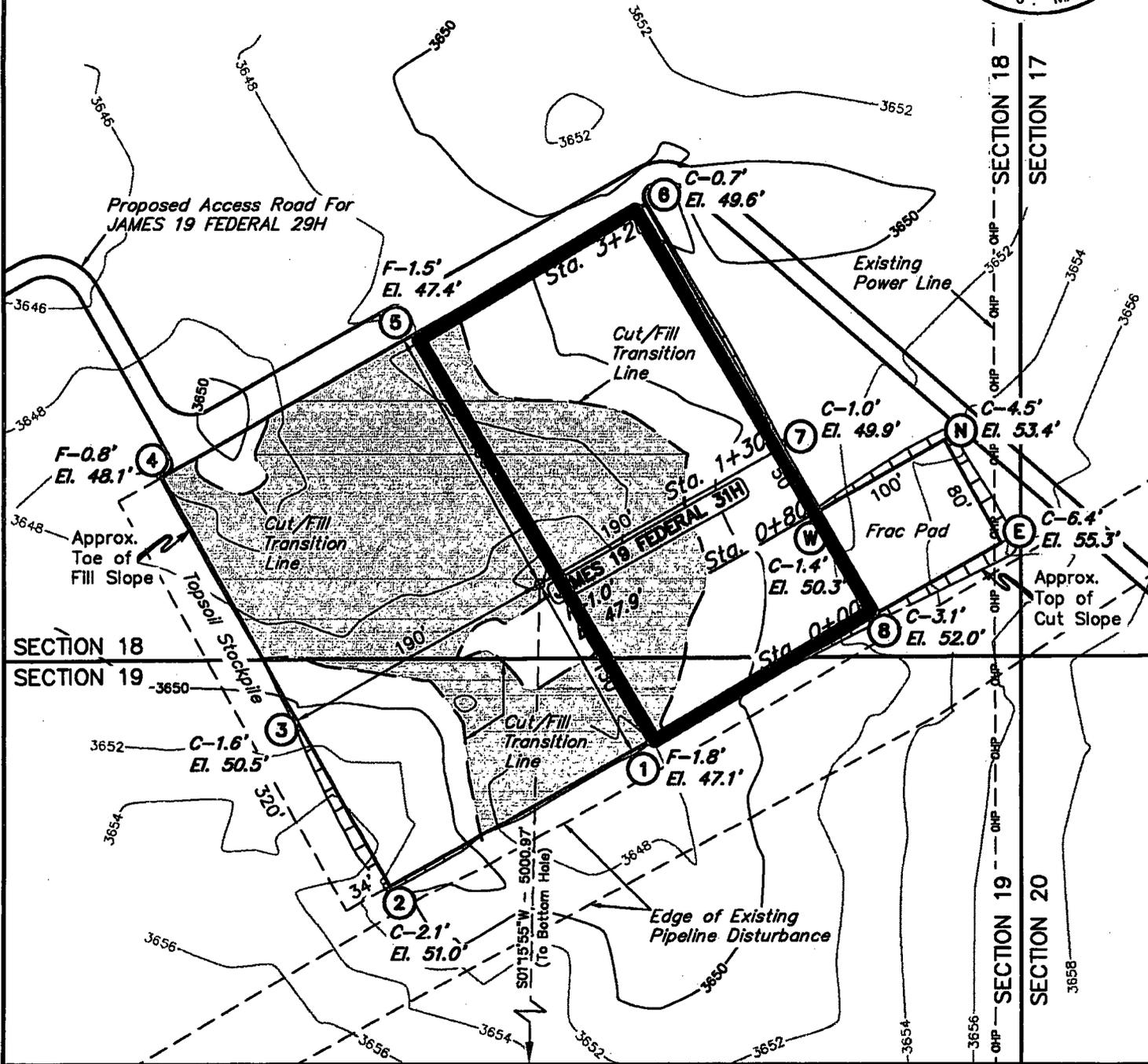
ELEV. UNGRADED GROUND AT LOC. STAKE = 3647.9' FINISHED GRADE ELEV. AT LOC. STAKE = 3648.9'
