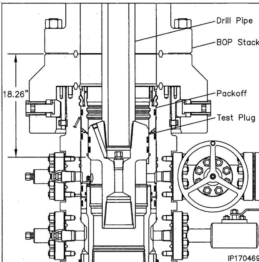
**Note:** Any leakage past the test plug will be clearly visible at the open side outlet valve.
