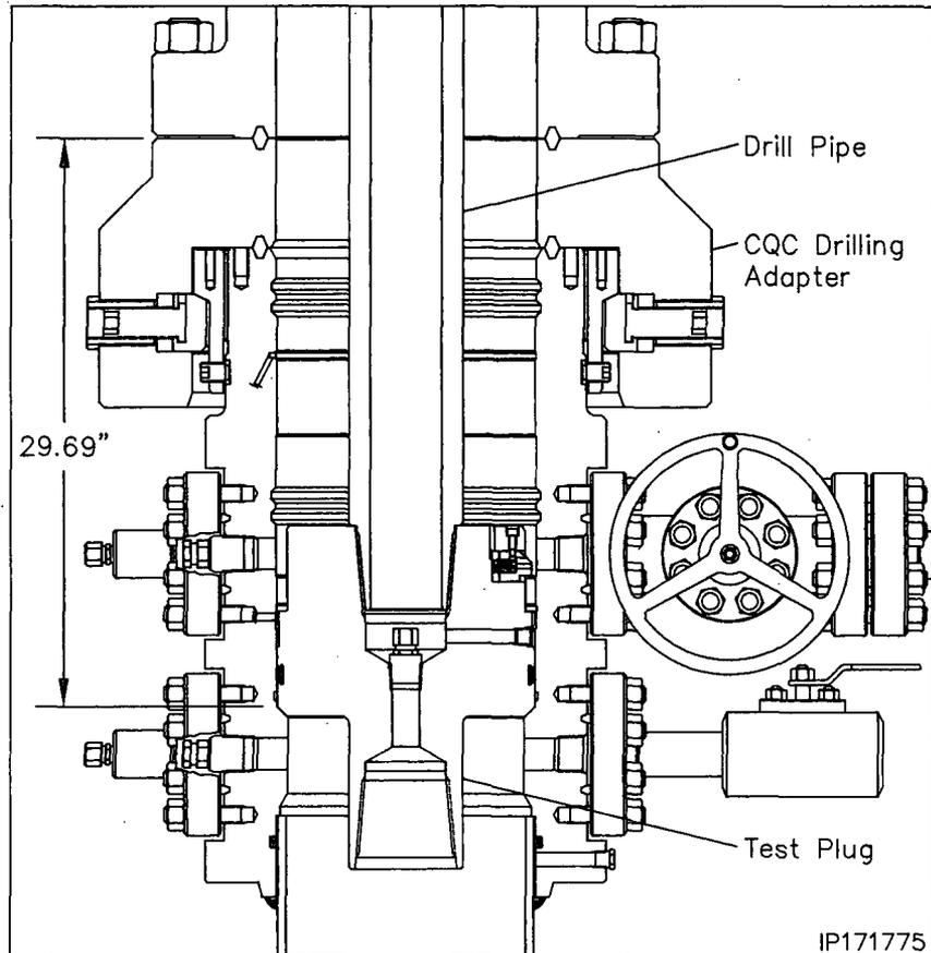
9. Remove as much fluid as possible from the BOP stack and the retrieve the test plug with a straight vertical lift.
