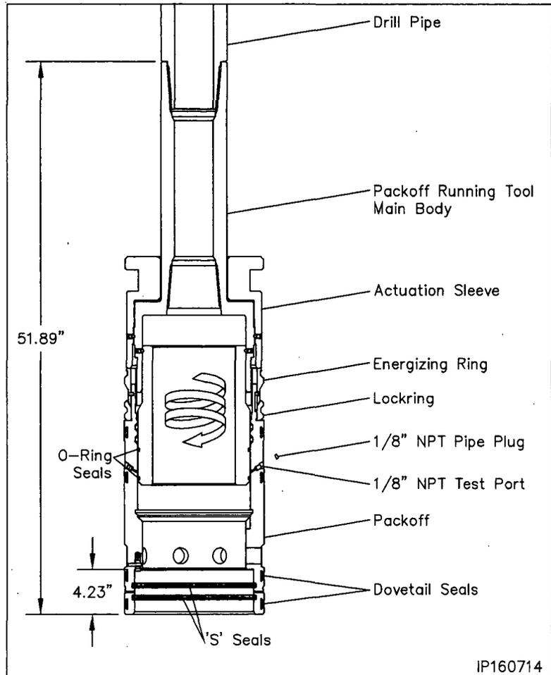
**WARNING:** All 1/8" pipe plugs must be removed prior to installing the packoff
