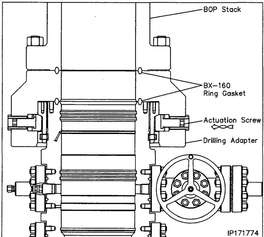
13. Ensure the BOP is level and then carefully run in all of the drive screws of the upper adapter to contact point.
