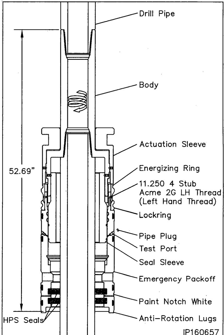
17. Using a straight edge positioned vertically and centered on the anti-rotation lug on the bottom of the packoff, place a white paint mark up the side of the packoff in line with the lug.
