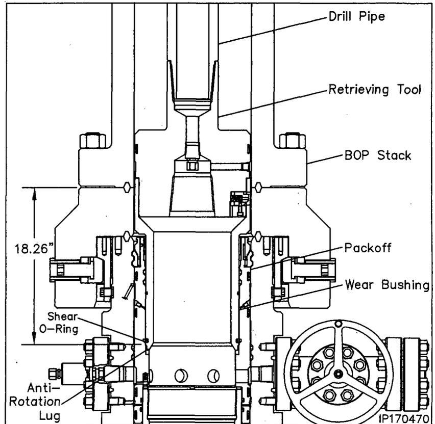
**Note:** The Shear O-Ring on bottom of the bushing will locate in a groove above the load shoulder in the head to act as a retaining device for the bushing.
