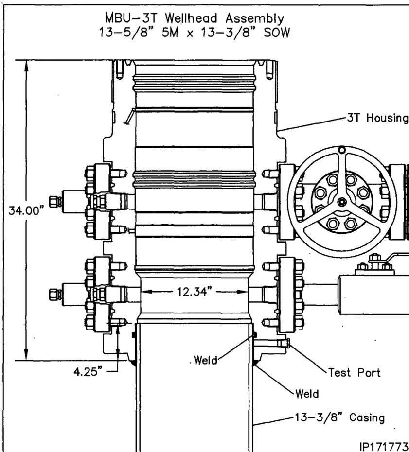
6. Align and level the Wellhead Assembly over the casing stub, orienting the outlets so they will be compatible with the drilling equipment.
