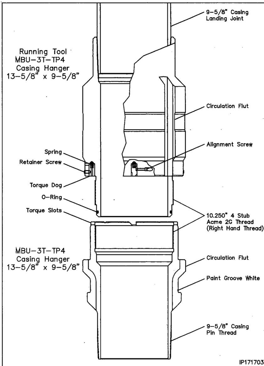
7. Calculate the total landing dimension by adding the previously determined RKB dimension and 29.69", the depth of the wellhead.
