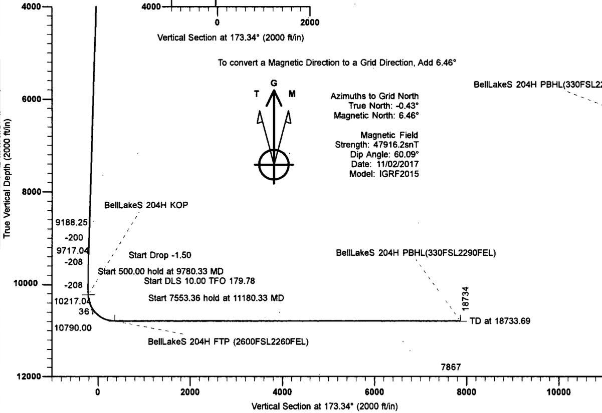
To convert a Magnetic Direction to a Grid Direction, Add 6.46°
