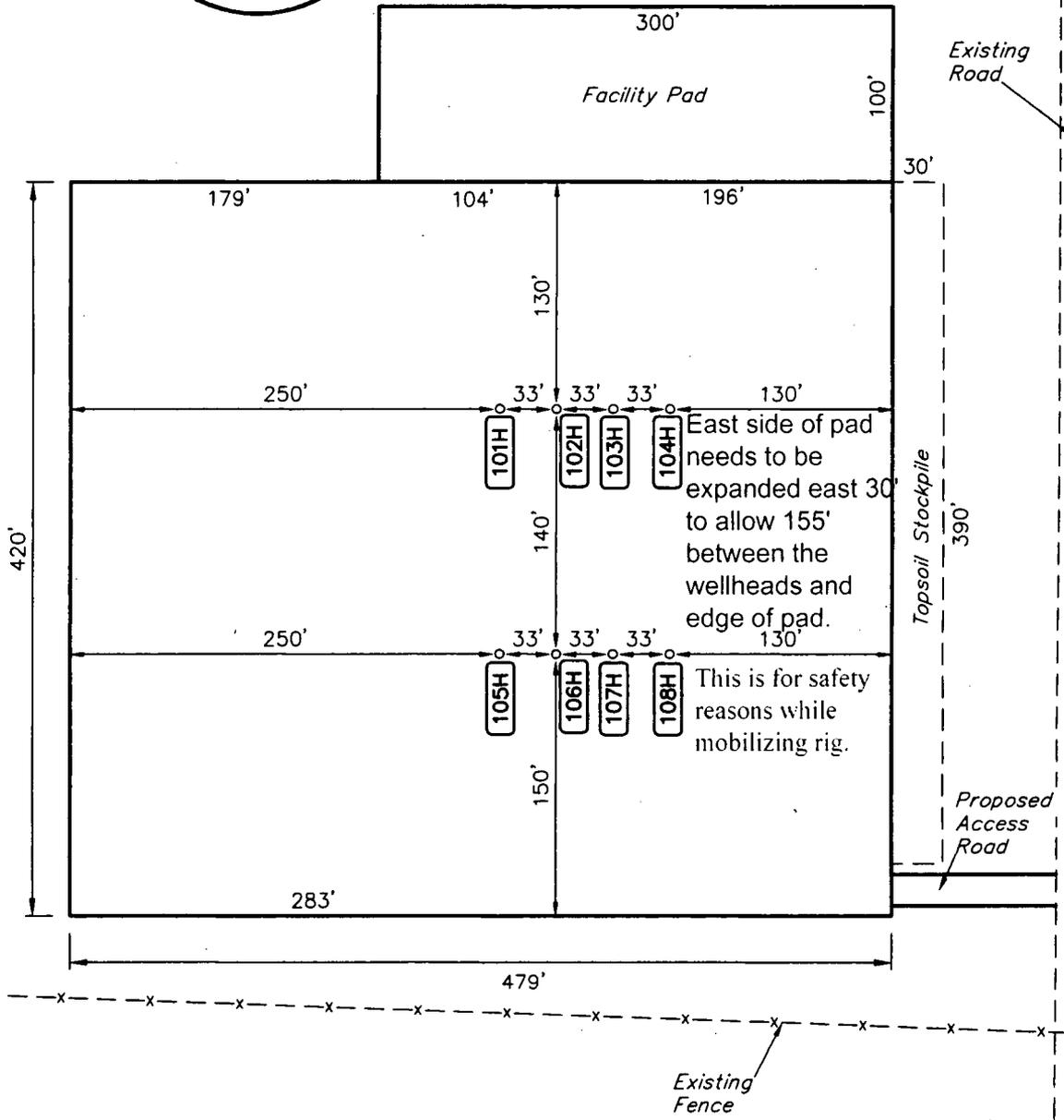
East side of pad needs to be expanded east 30' to allow 155' between the wellheads and edge of pad. This is for safety reasons while mobilizing rig.
