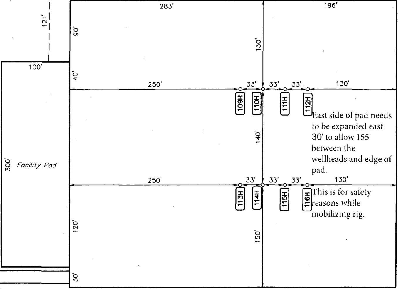
East side of pad needs to be expanded east 30' to allow 155' between the wellheads and edge of pad.
