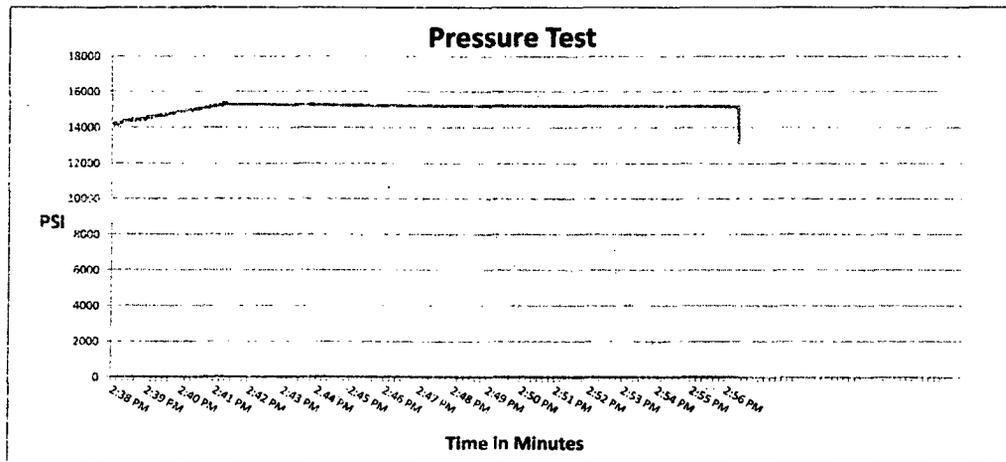
**Test Pressure** 15000 PSI      **Time Held at Test Pressure** 16 3/4 Minutes      **Actual Burst Pressure**      **Peak Pressure** 15410 PSI
