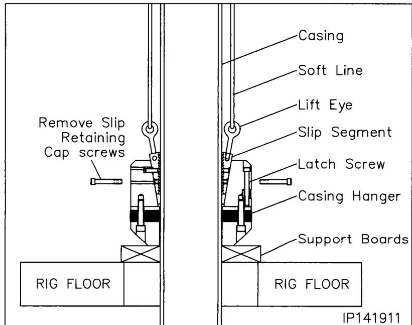
12. Slide the two hanger halves together ensuring the slip guide pins properly engage the opposing hanger half.
