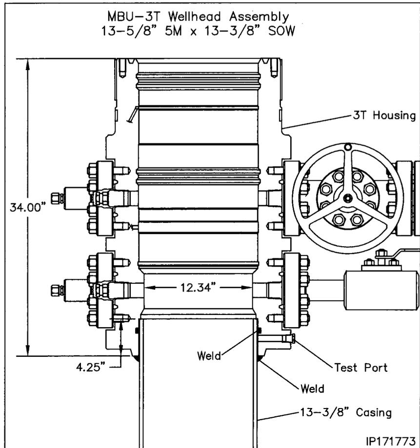
6. Align and level the Wellhead Assembly over the casing stub, orienting the outlets so they will be compatible with the drilling equipment.
