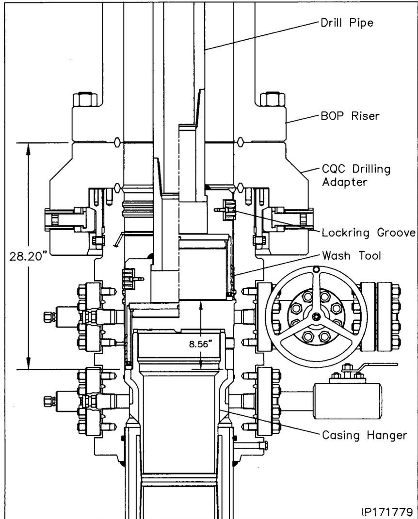
11. Reengage the pump and fully wash the inside of the wellhead and the entire BOP one additional cycle ensuring the stopping point is with the wash tool resting on top of the hanger flutes.
