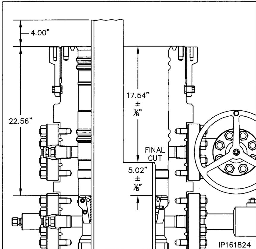
**Note:** There must not be any rough edges on the casing or the seals of the Packoff will be damaged.
