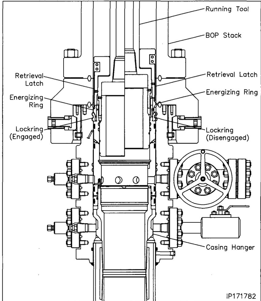
7. Carefully pick up on the drill pipe and remove the packoff from the MBU-3T wellhead with a straight vertical lift.
