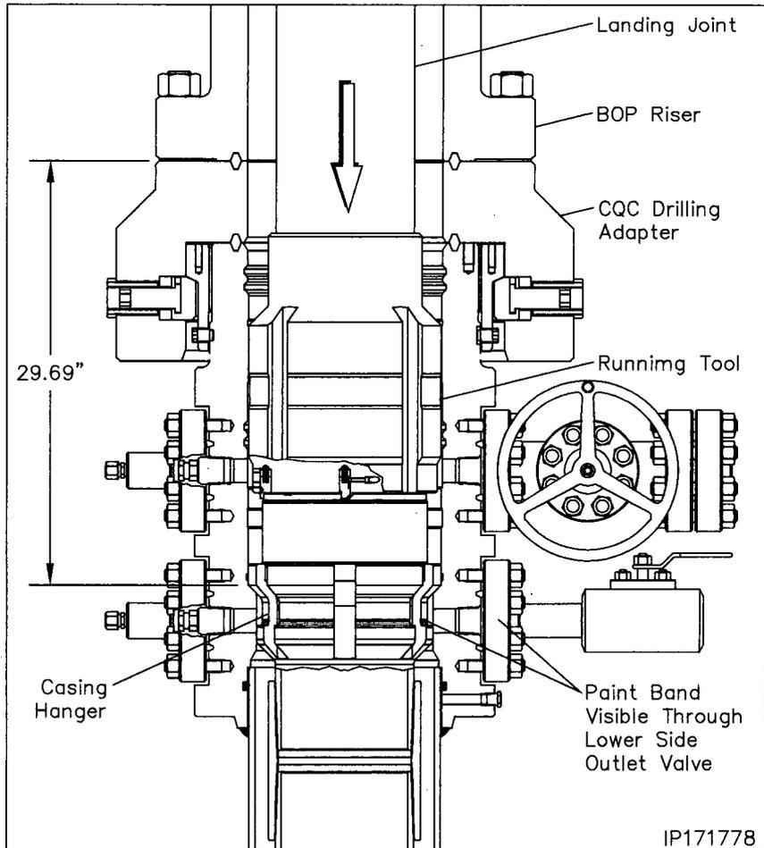
**Note:** Returns may be taken through the circulation slots and out the BOP or out the side outlets on the housing.
