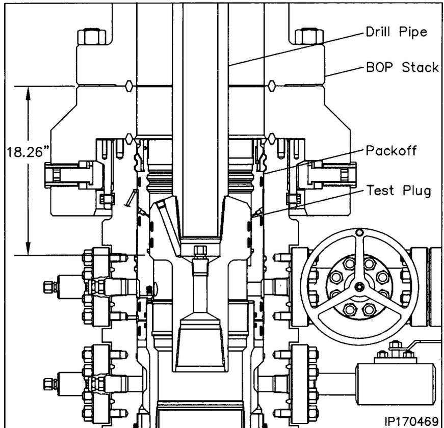
**Note:** Any leakage past the test plug will be clearly visible at the open side outlet valve.
