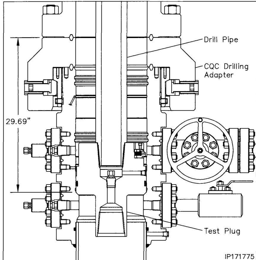
9. Remove as much fluid as possible from the BOP stack and retrieve the test plug with a straight vertical lift.
