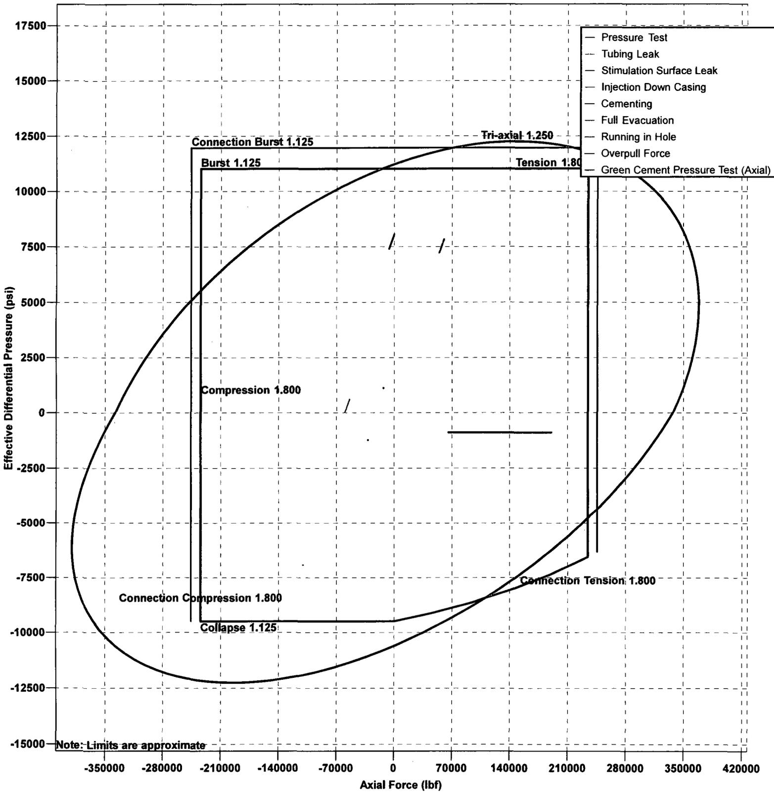
Design Limits (9 5/8" Intermediate Casing - Section 1)
