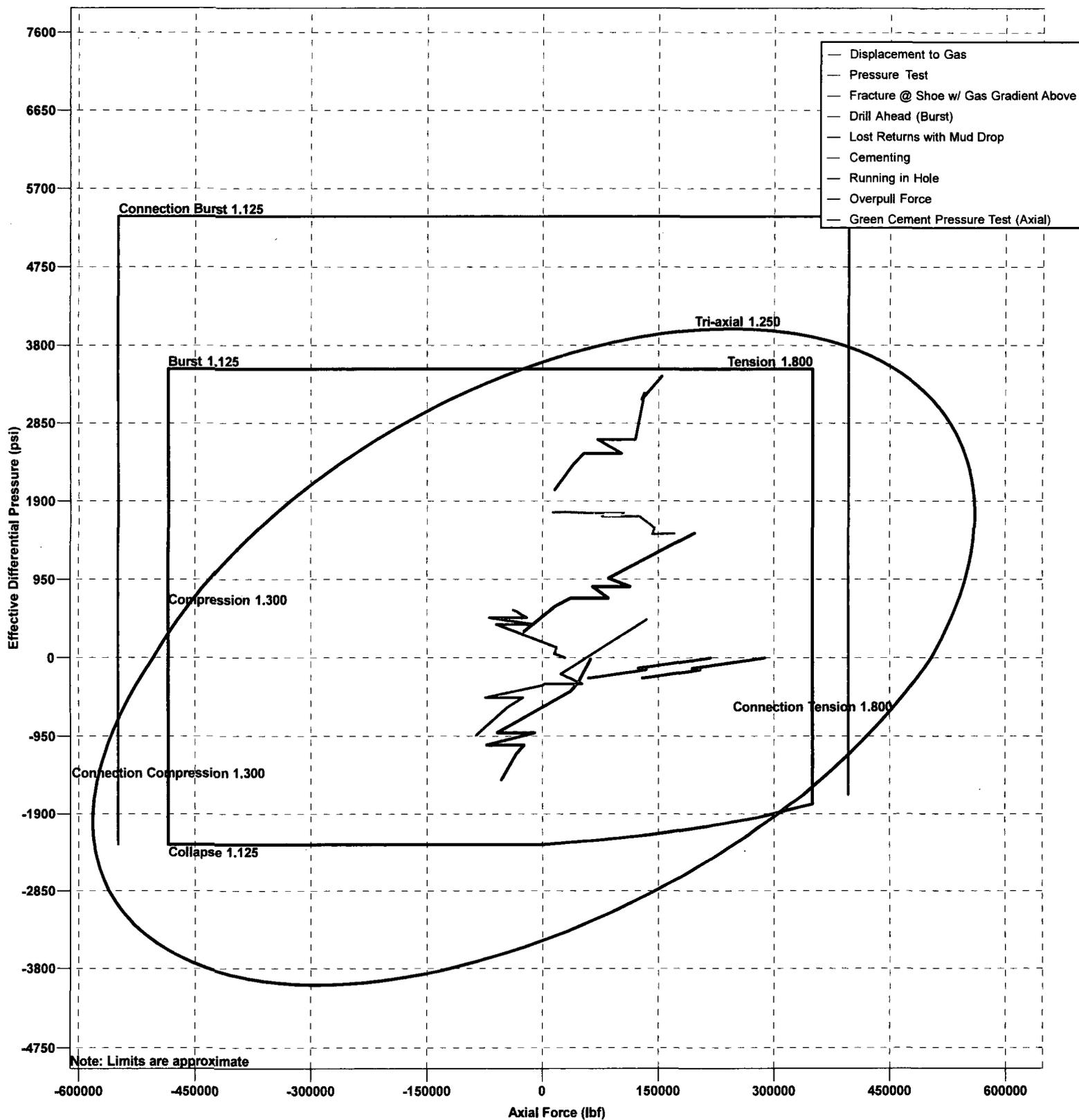
Design Limits (5 1/2" Production Casing - Section 1)
