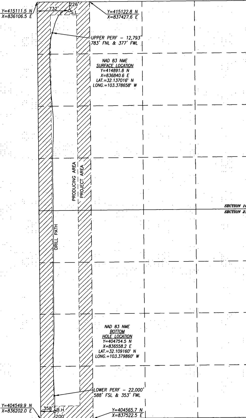
BOREPATH SHOWN HEREON IS BASED ON DIRECTIONAL SURVEY REPORT PROVIDED BY COG OPERATING, LLC FOR THE WHITE FALCON 16 ST COM #23H SUPPLIED TO HARCROW SURVEYING, LLC ON AUGUST 14, 2018
