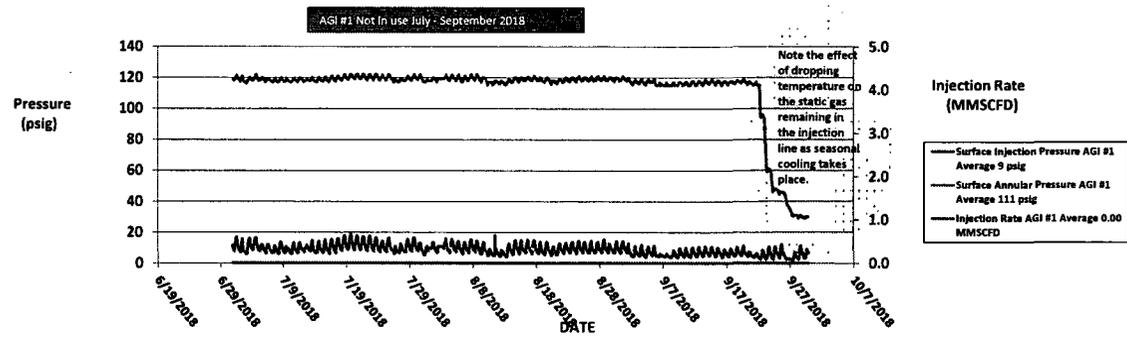
**FIGURE 3: ZIA AGI #1 SURFACE INJECTION PRESSURE, ANNULAR PRESSURE AND INJECTION TEMPERATURE**
