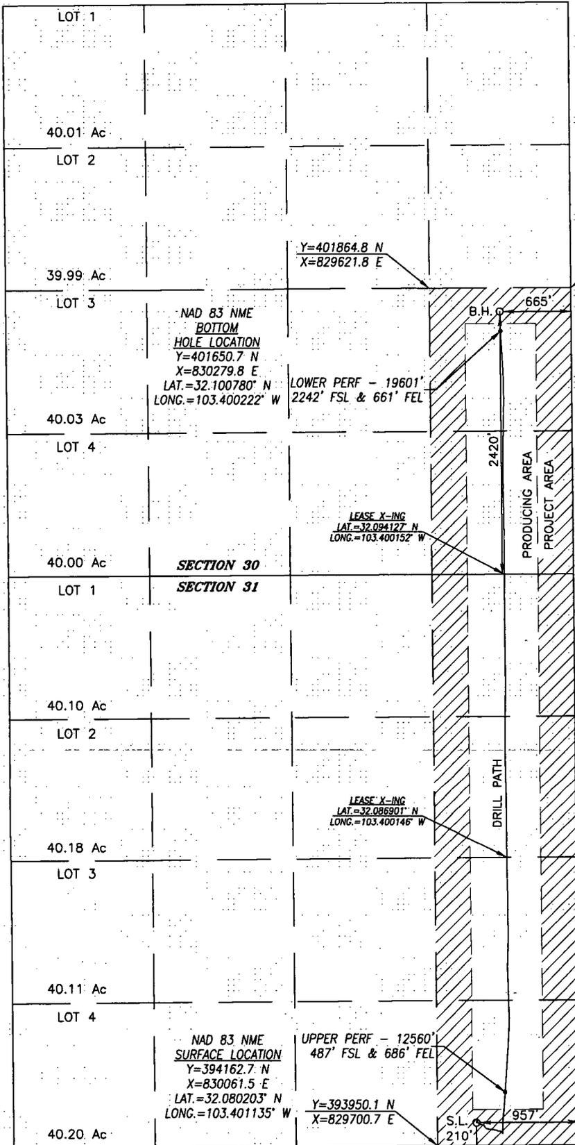
BOREPATH SHOWN HEREON IS BASED ON DIRECTIONAL SURVEY REPORT PROVIDED BY COG FOR THE SQUARE BILL FED COM #1H SUPPLIED TO HARCROW SURVEYING, LLC ON SEPTEMBER 21, 2018.
