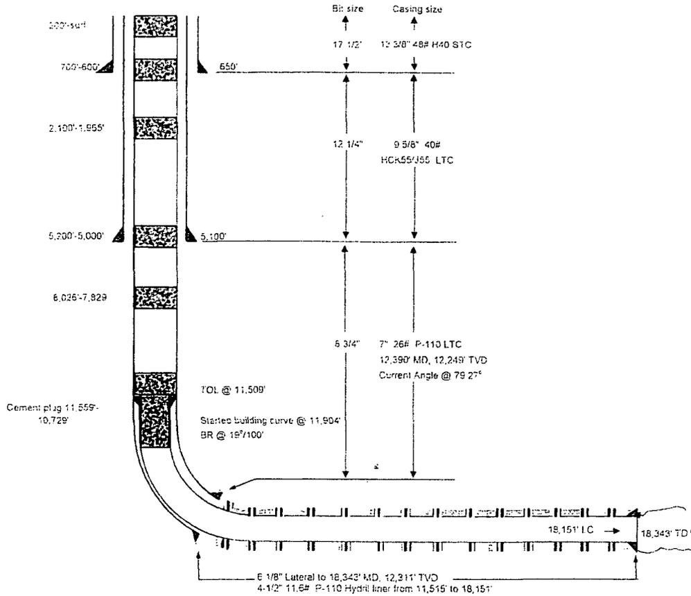
Perforate 4 1/2" liner with 16 sets of perforations, 1st stage, 16,100, 16,385, 16,670, 16,955, 17,240, 17,530, 17,820, 18110' = 47 holes
