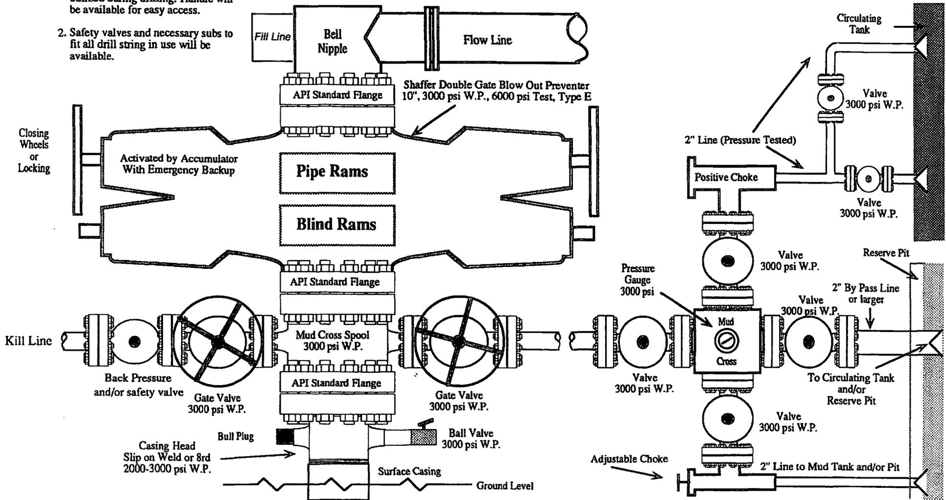
Note: This equipment is designed to meet requirements for a 2-M rating standard per 43 CFR part 3160 (amended). Proper operation and testing of equipment will be carried out per standard. 2,000 psi equipment can be substituted in the drawing to meet minimum requirements per standard.
