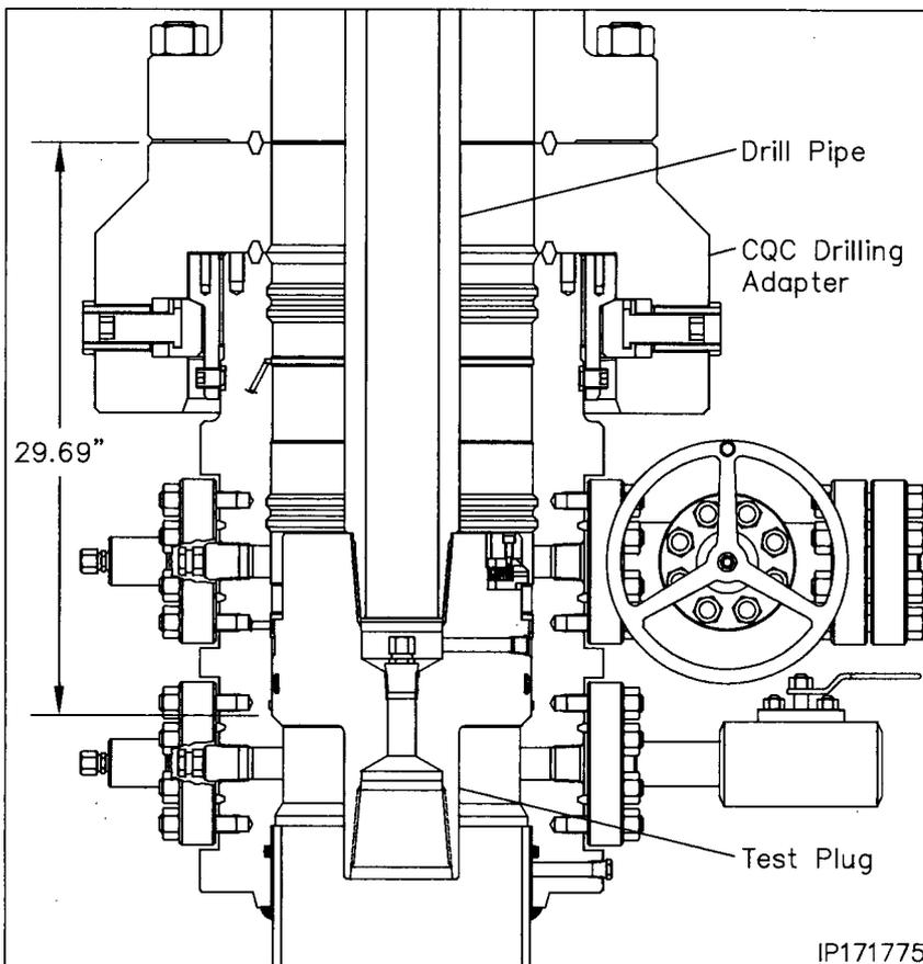
9. Remove as much fluid as possible from the BOP stack and retrieve the test plug with a straight vertical lift.
