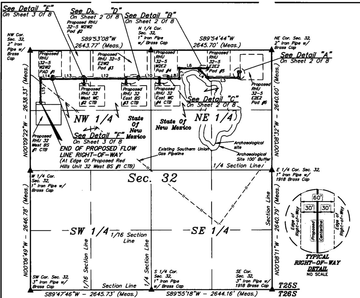
BEGINNING OF FLOW LINE BEARS S55°13'29"W 838.69' FROM THE NORTHEAST CORNER OF SECTION 32, T25S, R33E, N.M.P.M.
