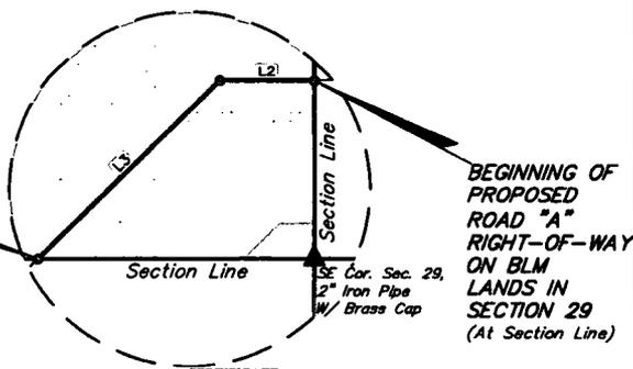
BEGINNING OF ROAD ON BLM LANDS IN SECTION 29 BEARS N00°07'52"W 18.61' FROM THE SOUTHEAST CORNER OF SECTION 29, T25S, R33E, N.M.P.M.
