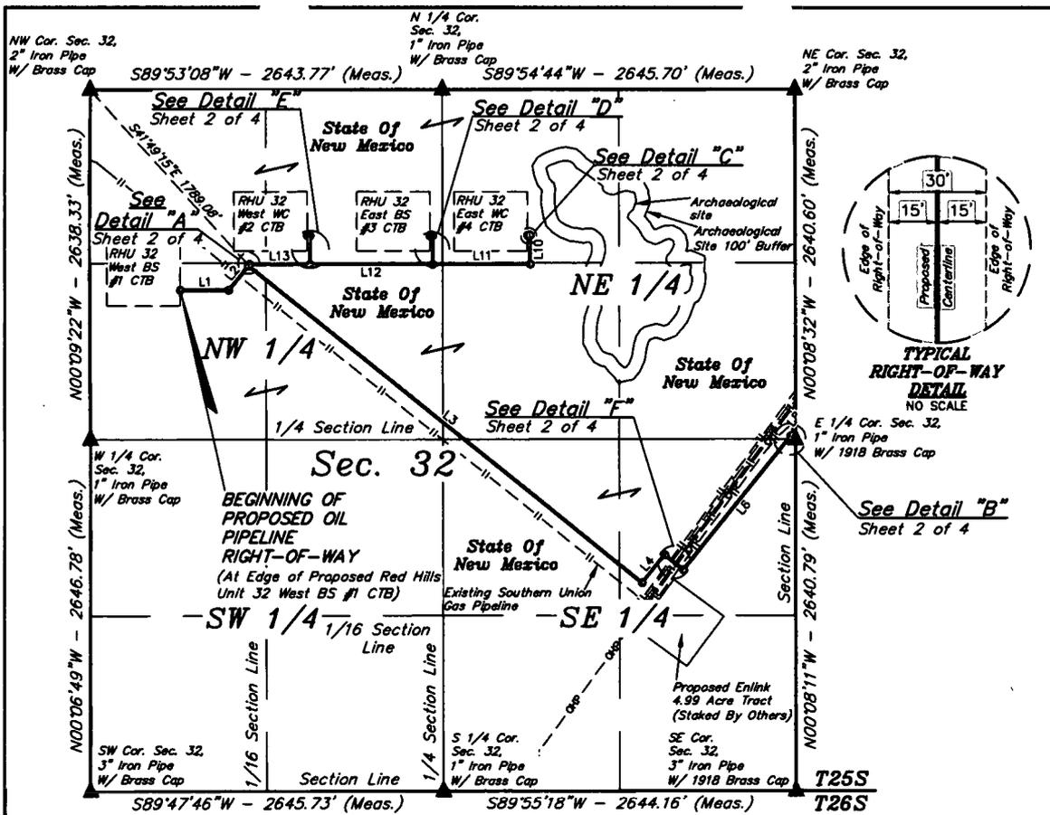
BEGINNING OF OIL PIPELINE BEARS N31°06'36"E 1309.85' FROM THE WEST 1/4 CORNER OF SECTION 32, T25S, R33E, N.M.P.M.
