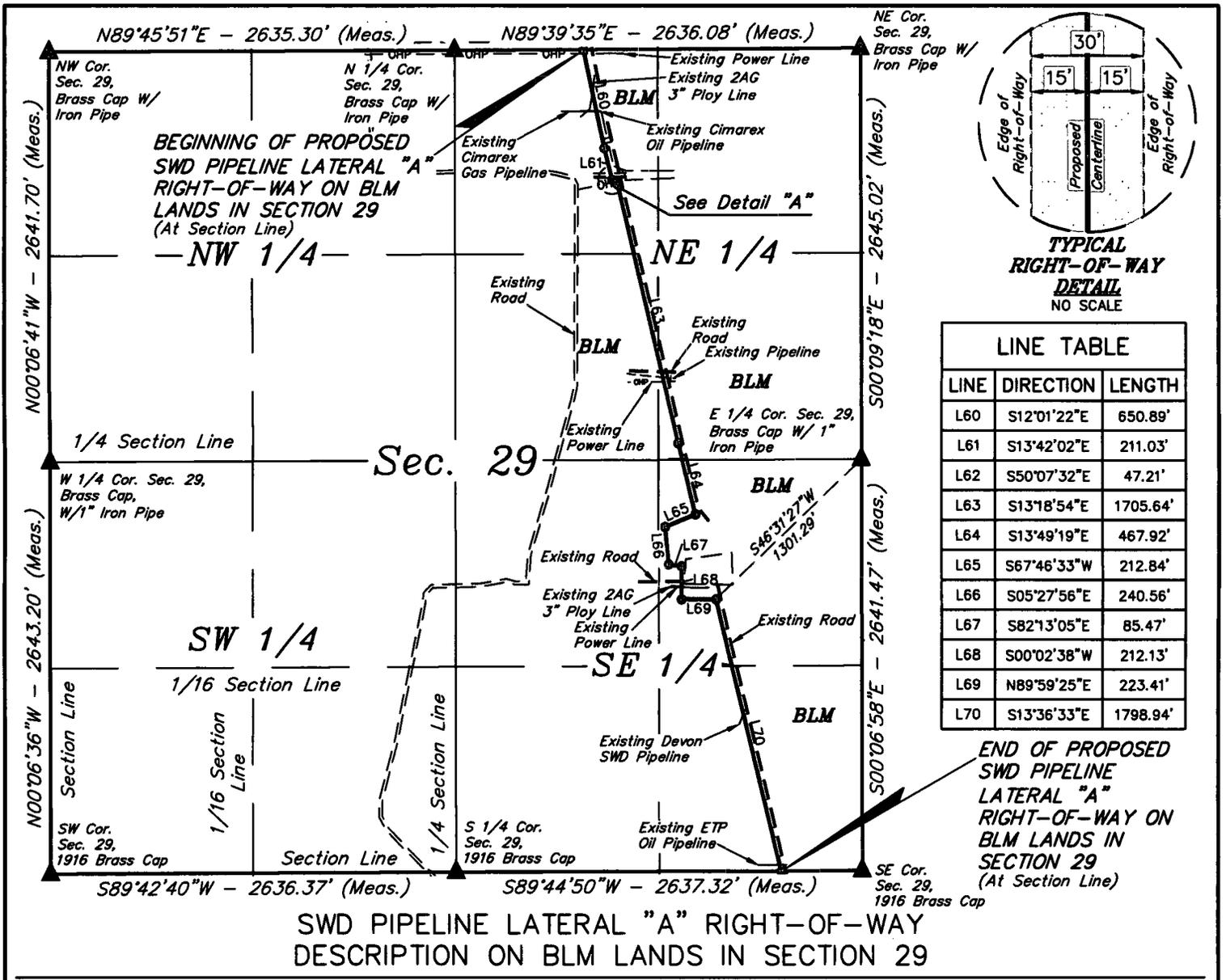
**SWD PIPELINE LATERAL "A" RIGHT-OF-WAY DESCRIPTION ON BLM LANDS IN SECTION 29**
