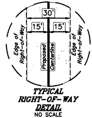
**SWD PIPELINE LATERAL "C" RIGHT-OF-WAY DESCRIPTION ON STATE OF NEW MEXICO LANDS IN SECTION 36**
