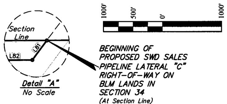
BEGINNING OF SWD SALES PIPELINE LATERAL "C" ON BLM LANDS IN SECTION 34 BEARS S89°41'31\"W 190.63' FROM THE NORTHWEST CORNER OF SECTION 34, T23S, R32E, N.M.P.M.
