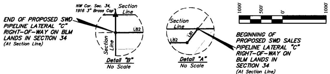
BEGINNING OF SWD SALES PIPELINE LATERAL "C" ON BLM LANDS IN SECTION 34 BEARS S89°41'31"W 190.63' FROM THE NORTHEAST CORNER OF SECTION 34, T23S, R32E, N.M.P.M.
