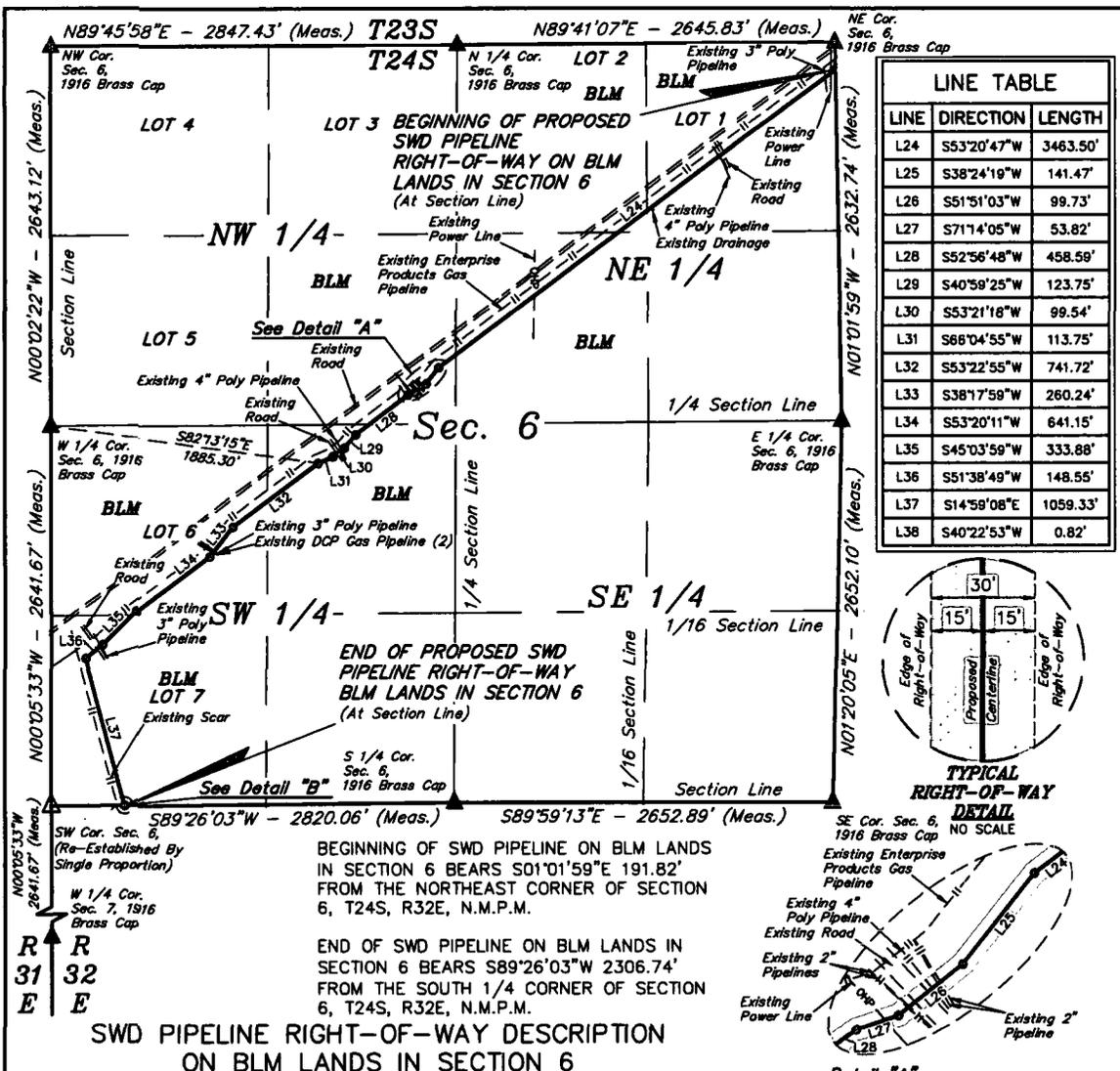
**BEGINNING OF SWD PIPELINE ON BLM LANDS IN SECTION 6 BEARS S01°01'59"E 191.82' FROM THE NORTHEAST CORNER OF SECTION 6, T24S, R32E, N.M.P.M.**
