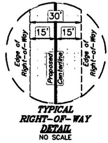
BEGINNING OF PROPOSED ACCESS ROAD RIGHT-OF-WAY ON BLM LANDS IN SECTION 19 (At Section Line)
