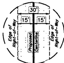
BEGINNING OF PROPOSED POWER LINE LATERAL "C" RIGHT-OF-WAY (At Proposed Power Line "B")
