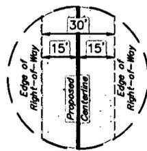
**BEGINNING OF PROPOSED ACCESS ROAD RIGHT-OF-WAY ON BLM LANDS IN SECTION 18 (At Section Line)**
