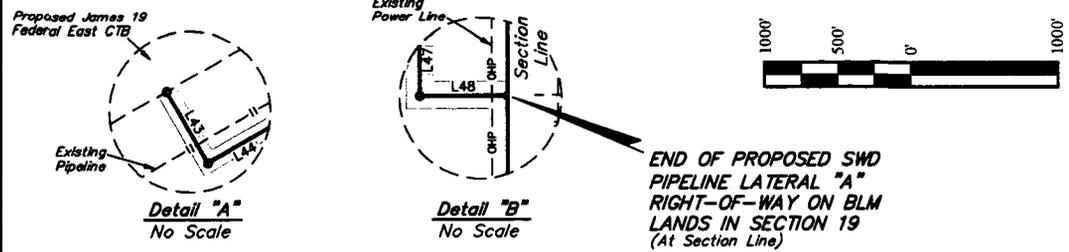
BEGINNING OF SWD PIPELINE LATERAL "A" BEARS S63°22'37"W 1803.65' FROM THE NORTHEAST CORNER OF SECTION 19, T23S, R32E, N.M.P.M.
