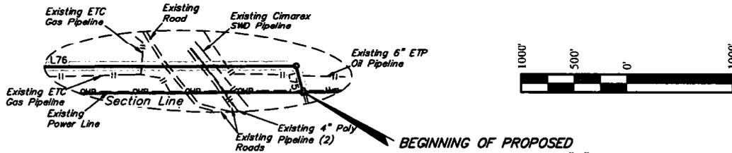
BEGINNING OF SWD PIPELINE LATERAL "C" ON BLM LANDS IN SECTION 25 BEARS N89°39'22"E 1100.36' FROM THE SOUTHWEST CORNER OF SECTION 25, T23S, R32E, N.M.P.M.
