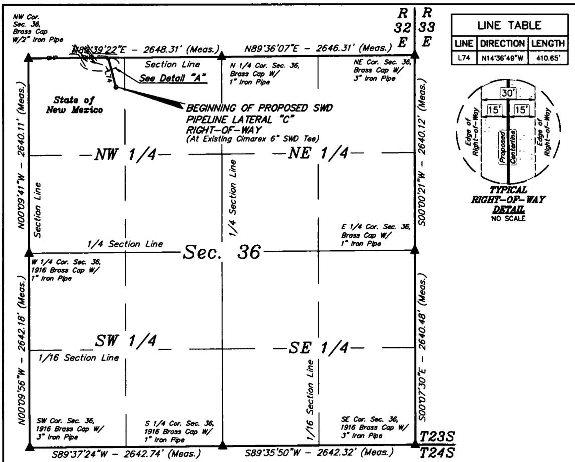
**SWD PIPELINE LATERAL "C" RIGHT-OF-WAY DESCRIPTION ON STATE OF NEW MEXICO LANDS IN SECTION 36**
