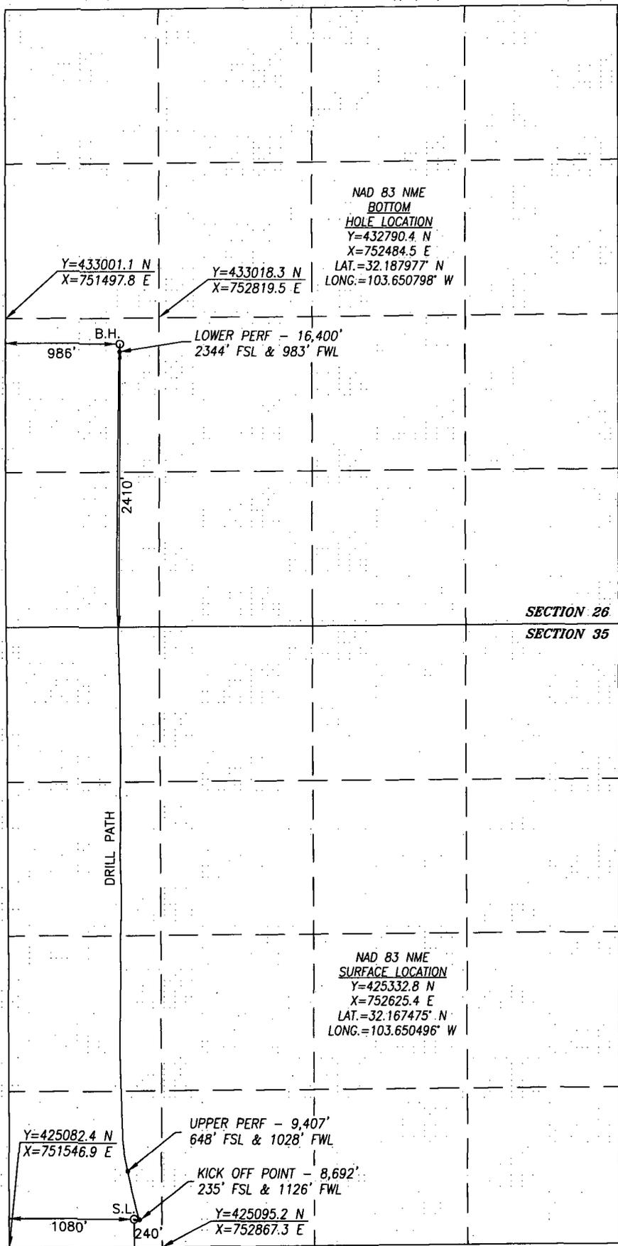
BOREPATH SHOWN HEREON IS BASED ON DIRECTIONAL SURVEY REPORT PROVIDED BY COG OPERATING, LLC FOR THE EIDER FEDERAL #102H SUPPLIED TO HARCROW SURVEYING, LLC ON FEBRUARY 4, 2019
