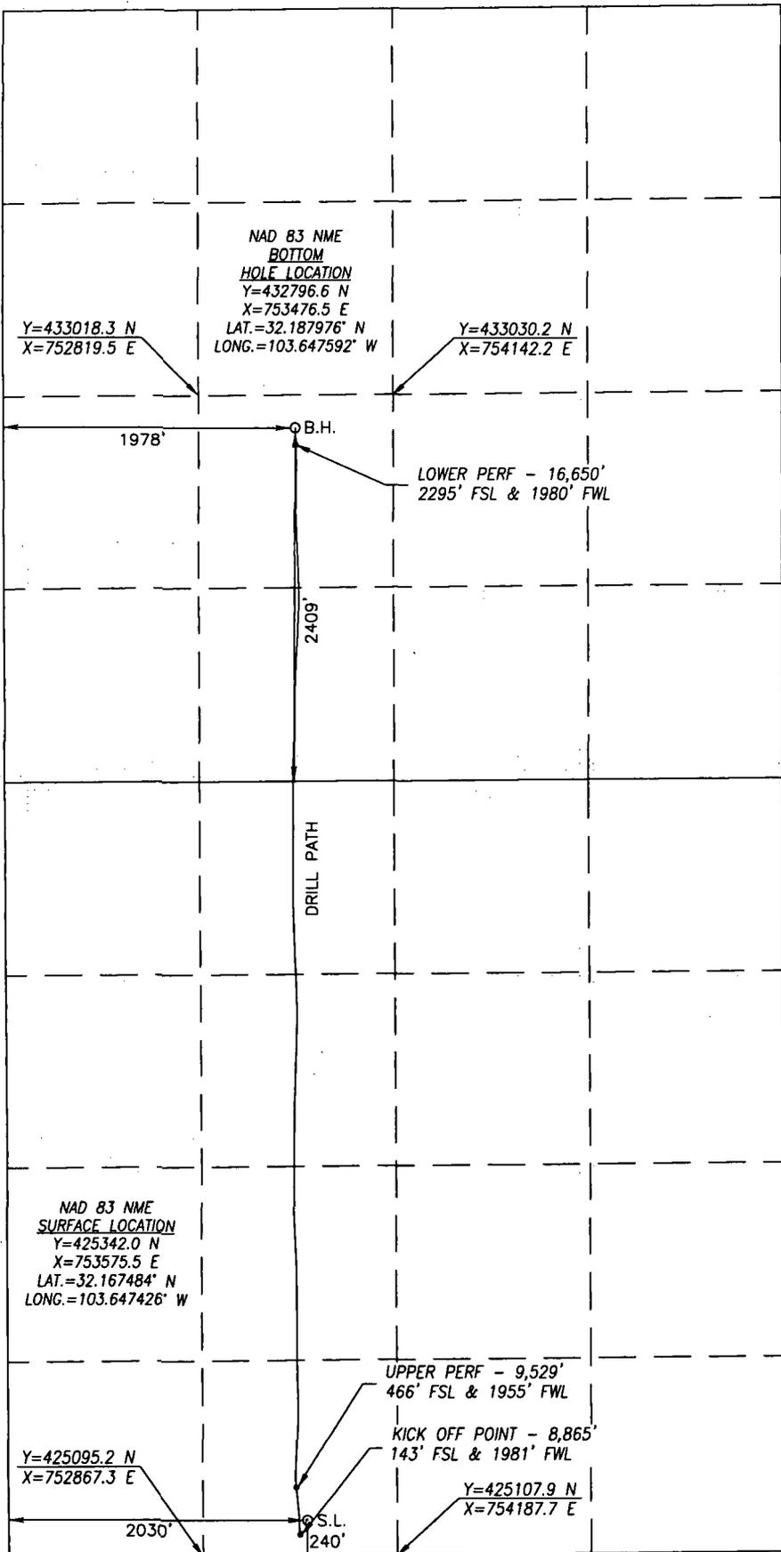
BOREPATH SHOWN HEREON IS BASED ON DIRECTIONAL SURVEY REPORT PROVIDED BY COG OPERATING, LLC FOR THE EIDER FEDERAL #203H SUPPLIED TO HARCROW SURVEYING, LLC ON JANUARY 29, 2019
