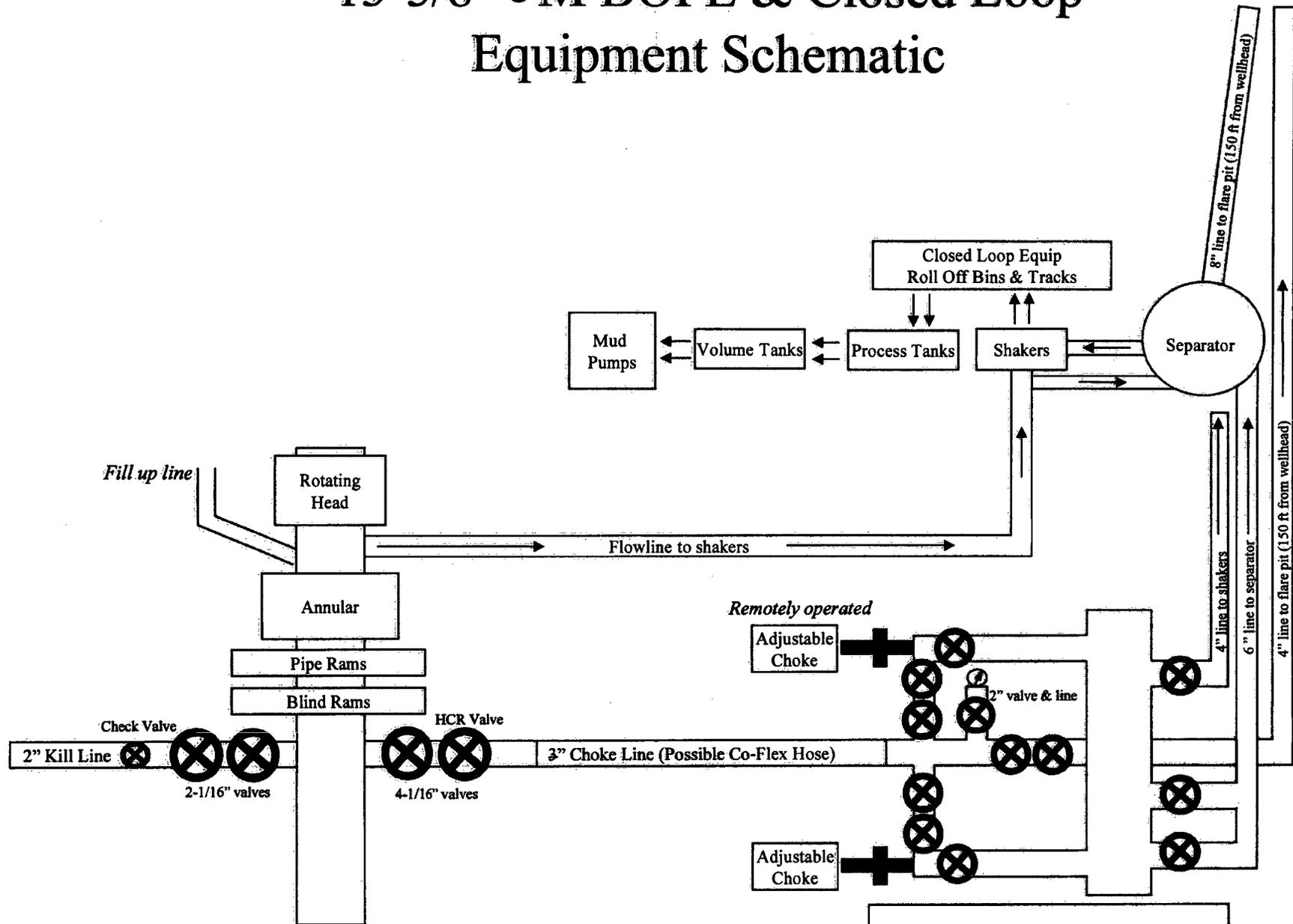
Note: all valves & lines on choke manifold are 3" unless otherwise noted. Exact manifold configuration may vary.
