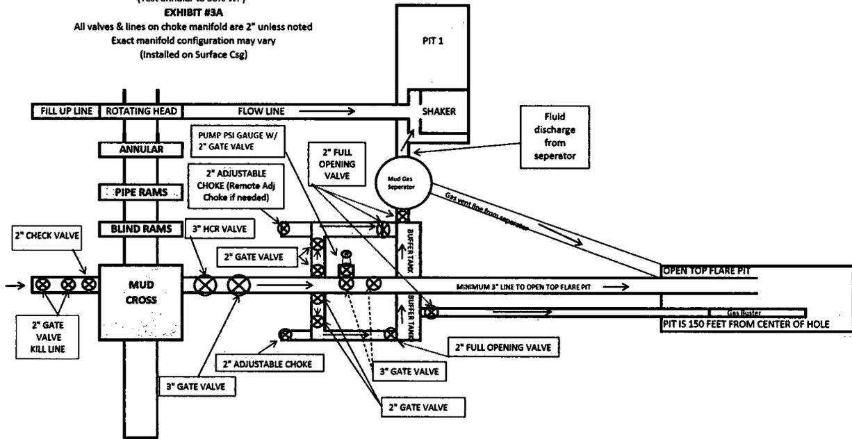
\*\*\* If H2S is encountered in quantities greater than 100ppm, Apache will shut in well & install a remote operated choke \*\*\*
