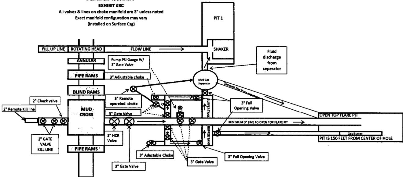
\*\*\* If H2S is encountered in quantities greater than 100ppm, Apache will shut in well & install a remote operated choke \*\*\*
