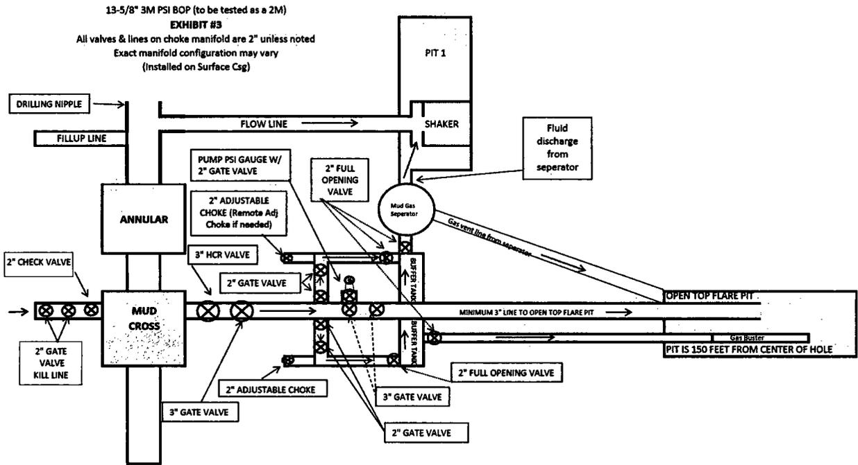
\*\*\* If H2S is encountered in quantities greater than 100ppm, Apache will shut in well & install a remote operated choke \*\*\*
