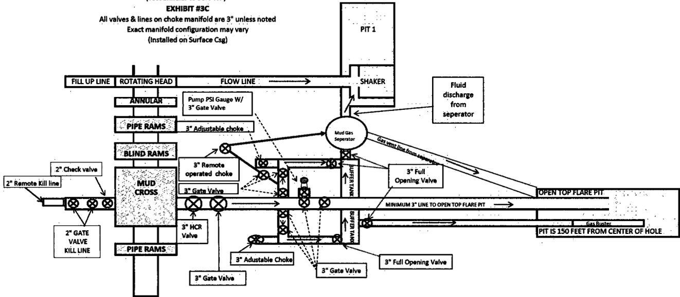
\*\*\* If H2S is encountered in quantities greater than 100ppm, Apache will shut in well & install a remote operated choke \*\*\*
