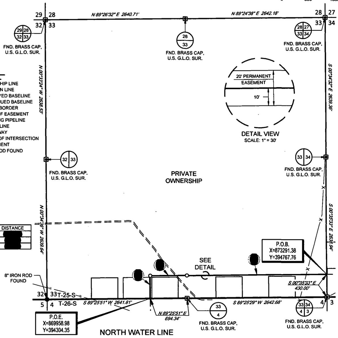
Being a proposed water line easement being 20 feet in width, 10 feet left and right of the above platted centerline total line footage containing 3766.78 feet or 228.29 rods, containing 1.73 acres more or less.
