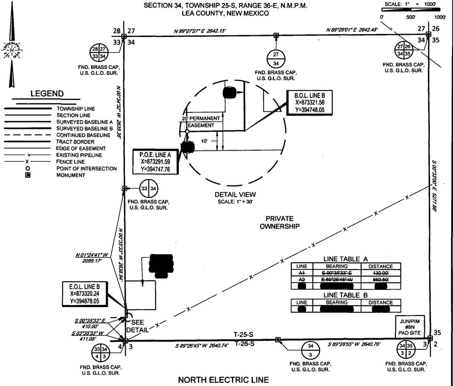
Being a proposed electric line easement being 20 feet in width, 10 feet left and right of the above platted centerline total line footage containing 830.00 feet or 50.30 rods, containing 0.38 acres more or less.
