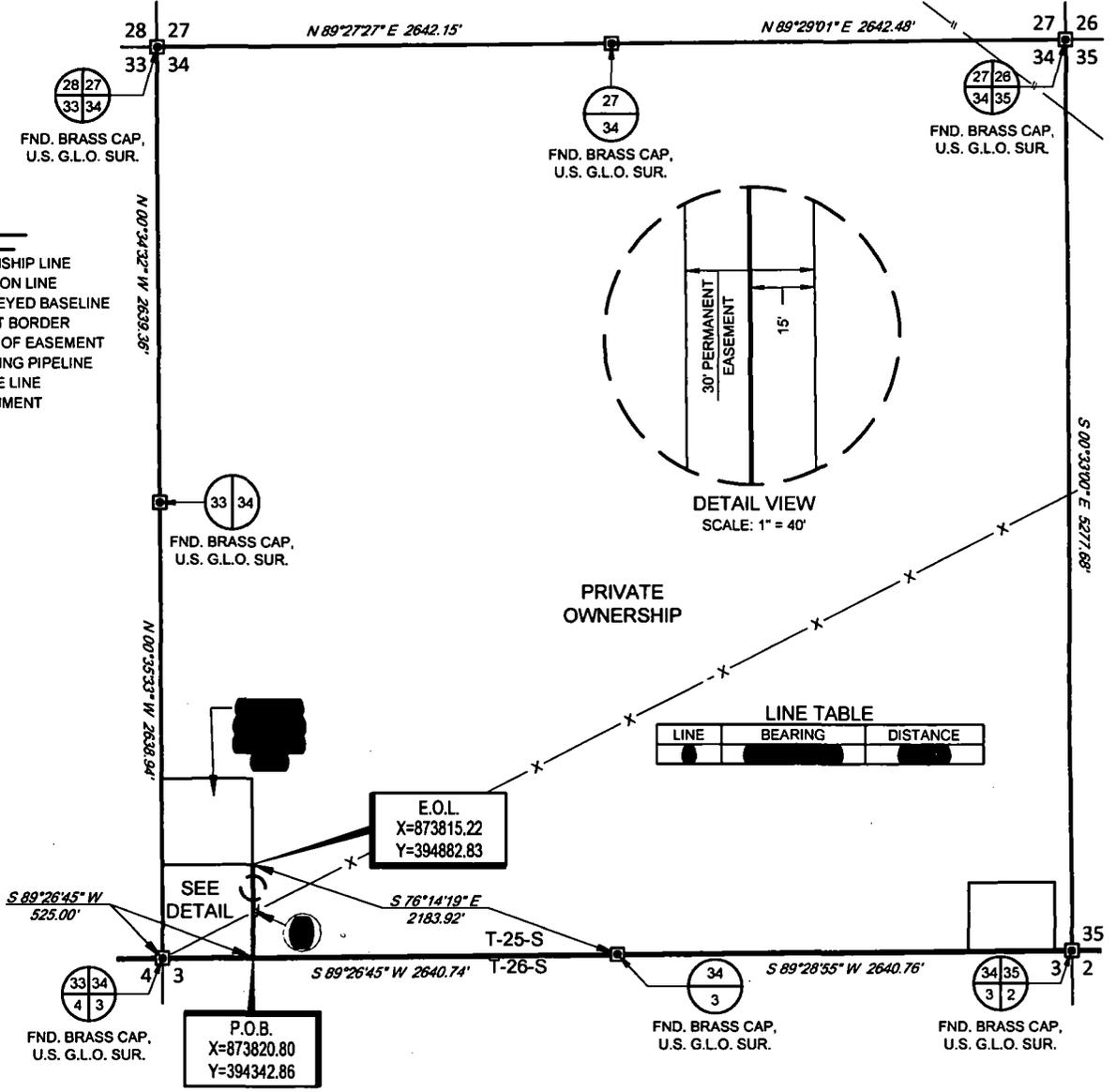
Being a proposed road easement being 30 feet in width, 15 feet left and right of the above platted centerline total line footage containing 540.00 feet or 32.73 rods, containing 0.37 acres more or less.
