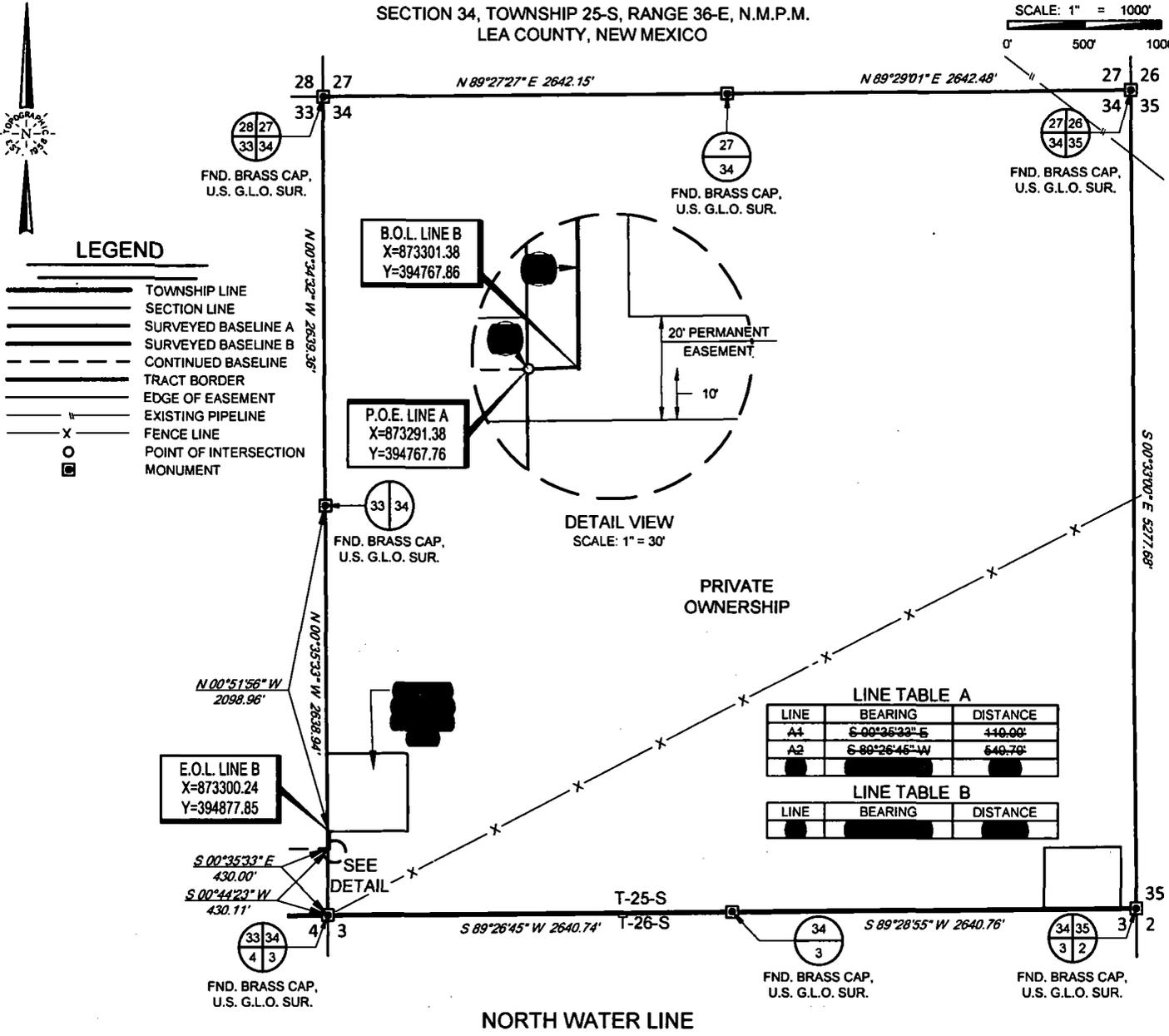
Being a proposed water line easement being 20 feet in width, 10 feet left and right of the above platted centerline total line footage containing 770.00 feet or 46.67 rods, containing 0.35 acres more or less.
