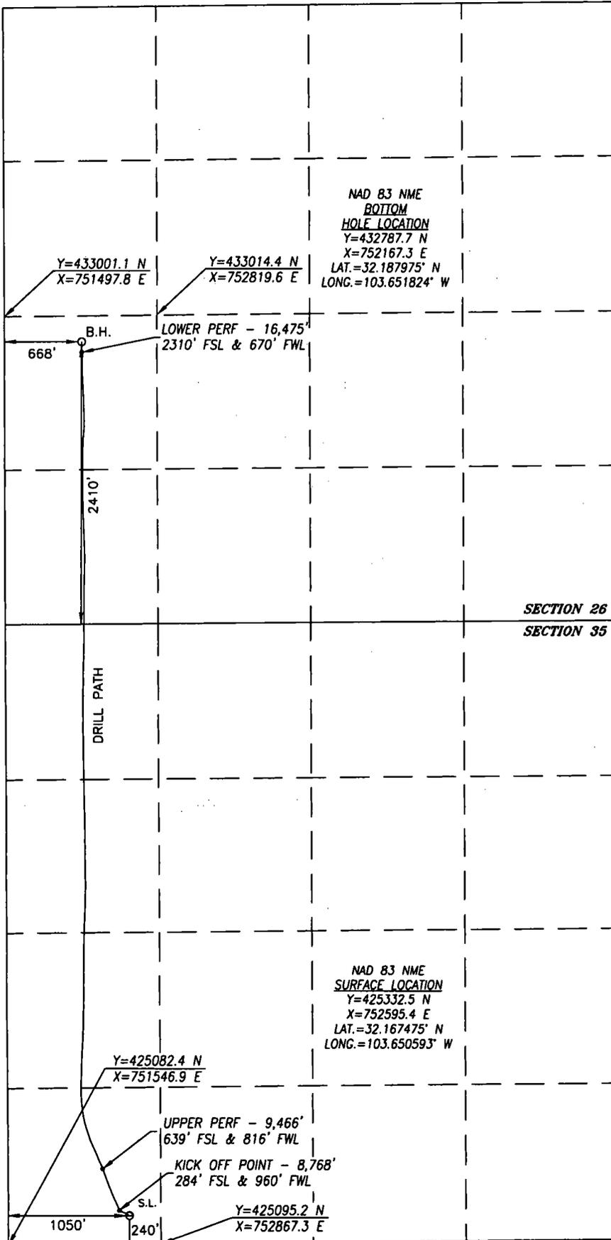
BOREPATH SHOWN HEREON IS BASED ON DIRECTIONAL SURVEY REPORT PROVIDED BY COG PRODUCTION, LLC FOR THE EIDER FEDERAL #201H SUPPLIED TO HARCROW SURVEYING, LLC ON JANUARY 28, 2018
