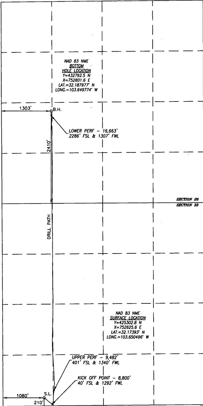
BOREPATH SHOWN HEREON IS BASED ON DIRECTIONAL SURVEY REPORT PROVIDED BY COG PRODUCTION, LLC FOR THE EIDER FEDERAL #202H SUPPLIED TO HARCROW SURVEYING, LLC ON MARCH 26, 2019
