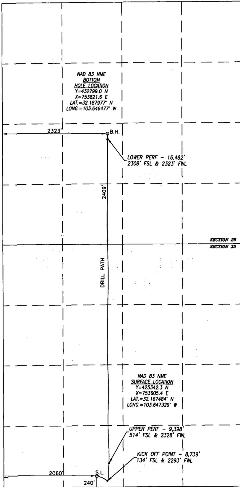
BOREPATH SHOWN HEREBON IS BASED ON DIRECTIONAL SURVEY REPORT PROVIDED BY COG PRODUCTION, LLC FOR THE EIDER FEDERAL #104H SUPPLIED TO HARCROW SURVEYING, LLC ON MARCH 28, 2019
