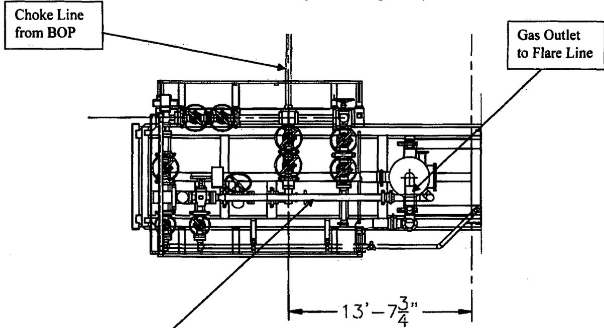
**Choke Manifold – Gas Separator (Side View)**
