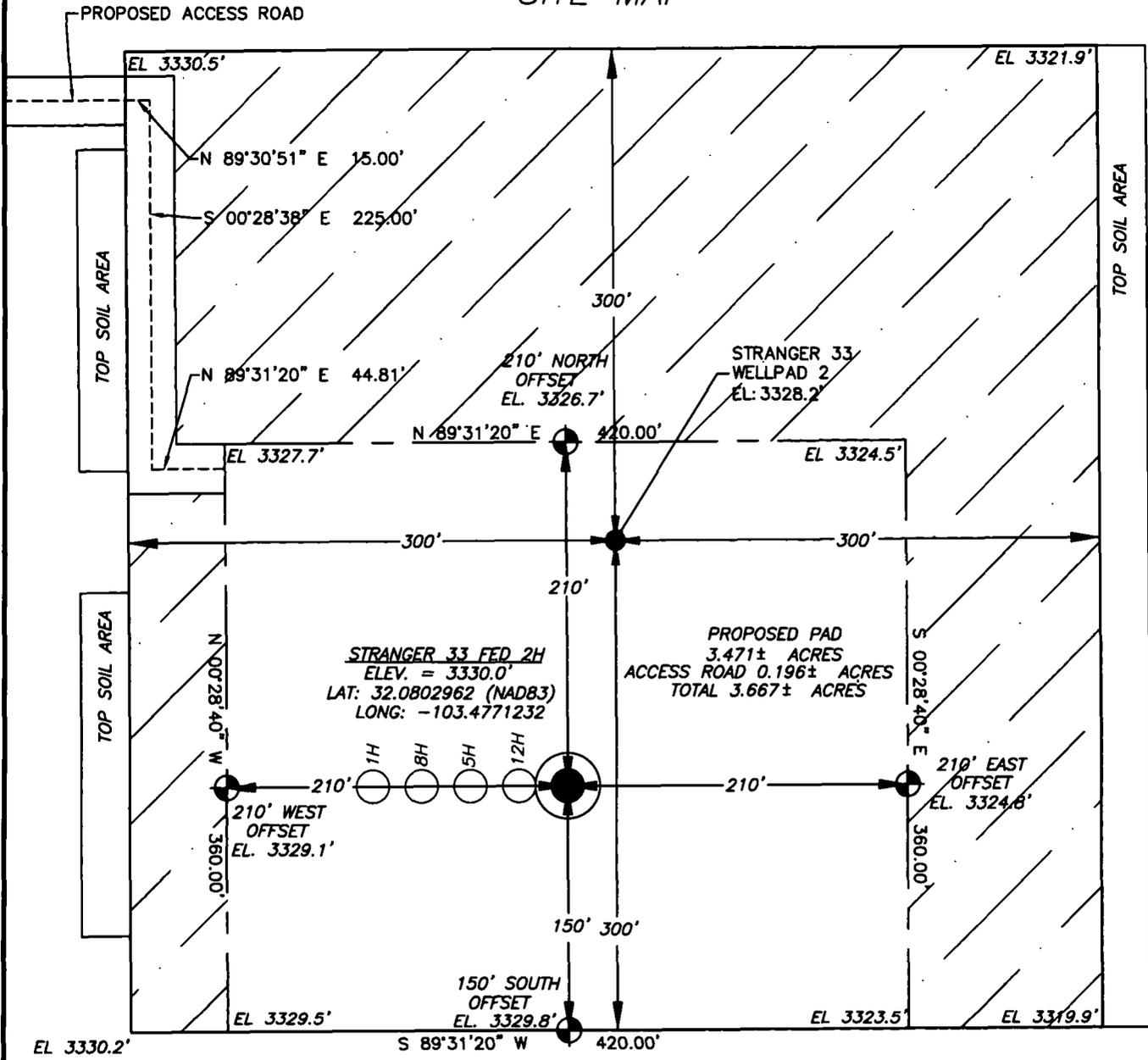
Note: All bearings recited herein are based on the New Mexico State Plane Coordinate System, NAD 83, New Mexico East Zone 3001, US Survey Feet, all distances are grid.
