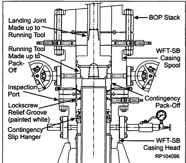
11. Verify, through inspection port that the pack-off bushing has landed properly after:
