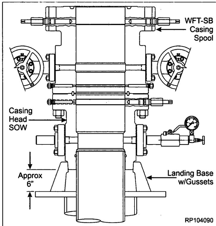
10. Determine the correct elevation for the wellhead assembly. Measure depth of the surface casing socket in SOW with O-ring bottom prep.
