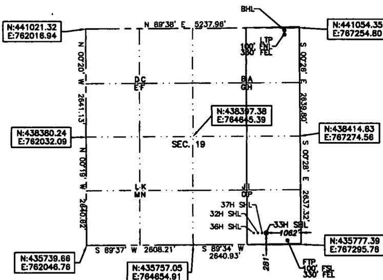
Note: All bearings recited herein are based on the New Mexico State Plane Coordinate System, NAD 83, New Mexico East Zone 3001, US Survey Feet, all distances are grid.
