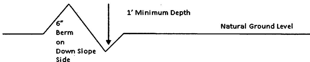
All lead-off ditches shall be graded to drain water with a 1 percent minimum to 3 percent maximum ditch slope. The spacing interval are variable for lead-off ditches and shall be determined according to the formula for spacing intervals of lead-off ditches, but may be amended depending upon existing soil types and centerline road slope (in %);
