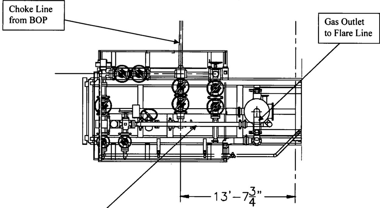
**Choke Manifold – Gas Separator (Side View)**
