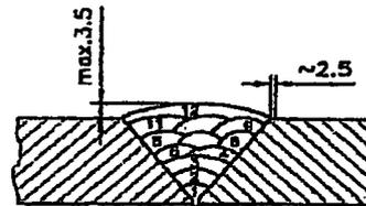
Groove Design for Test Coupon
