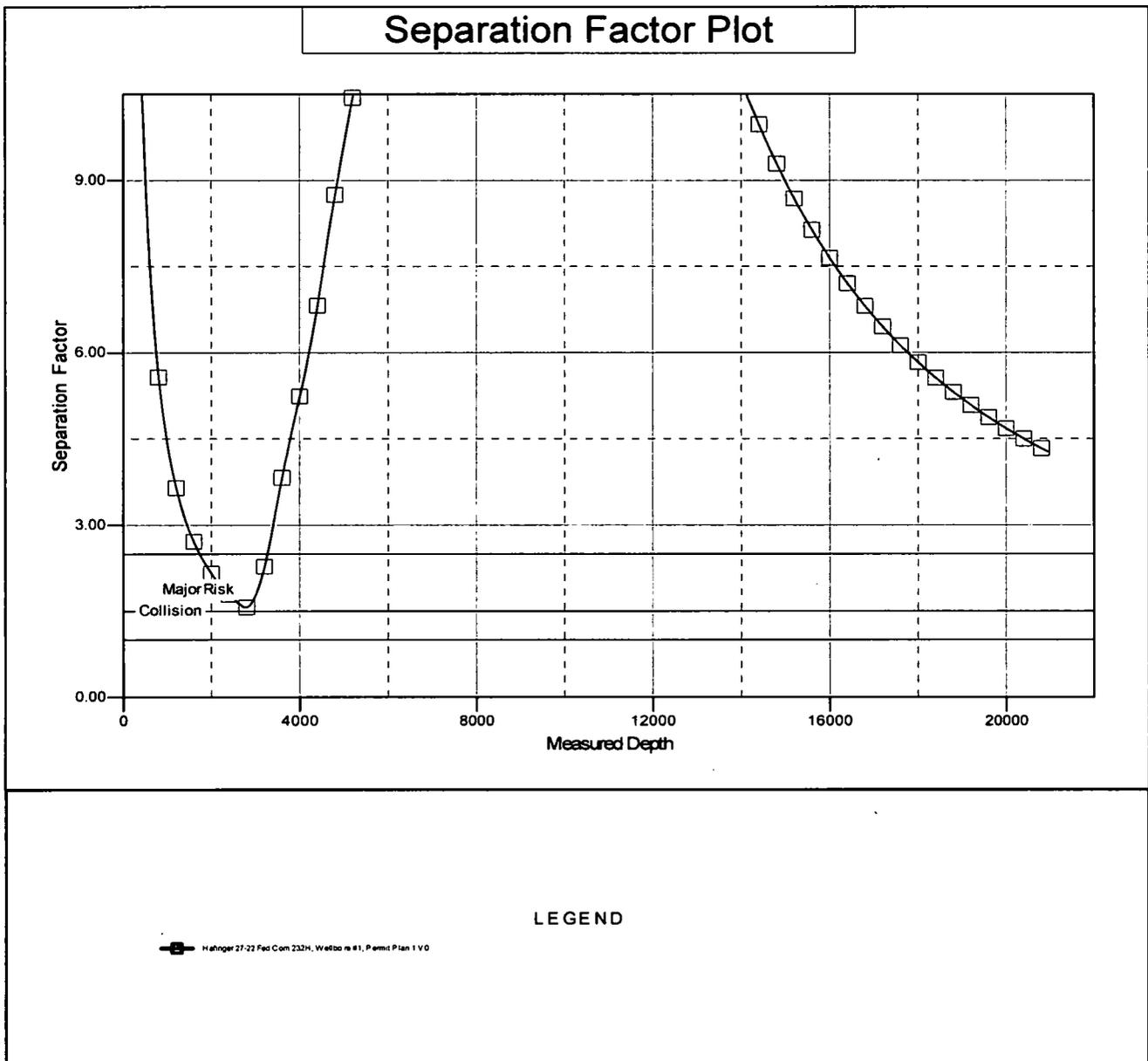
CC - Min centre to center distance or convergent point, SF - min separation factor, ES - min ellipse separation
