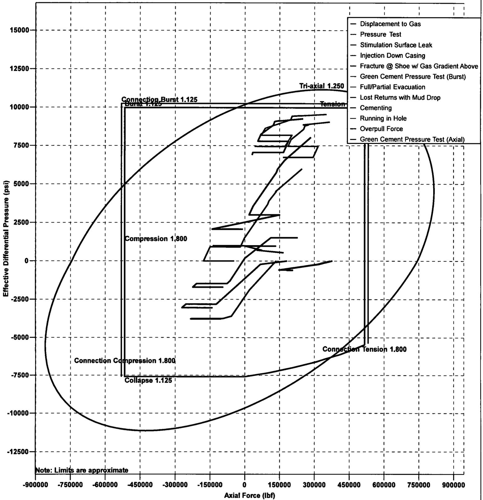
**Design Limits (13 3/8" Surface Casing - Section 1)**
