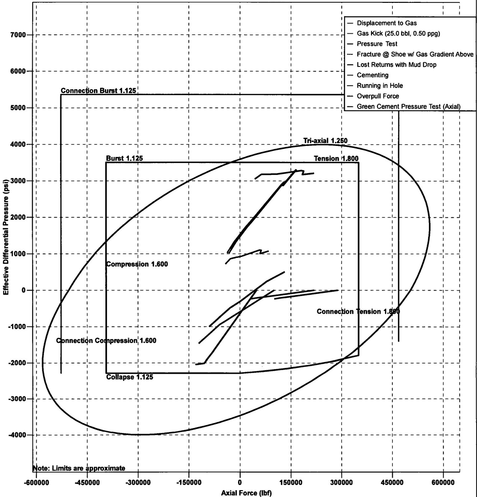
Design Limits (9 5/8" Intermediate Casing - Section 1)
