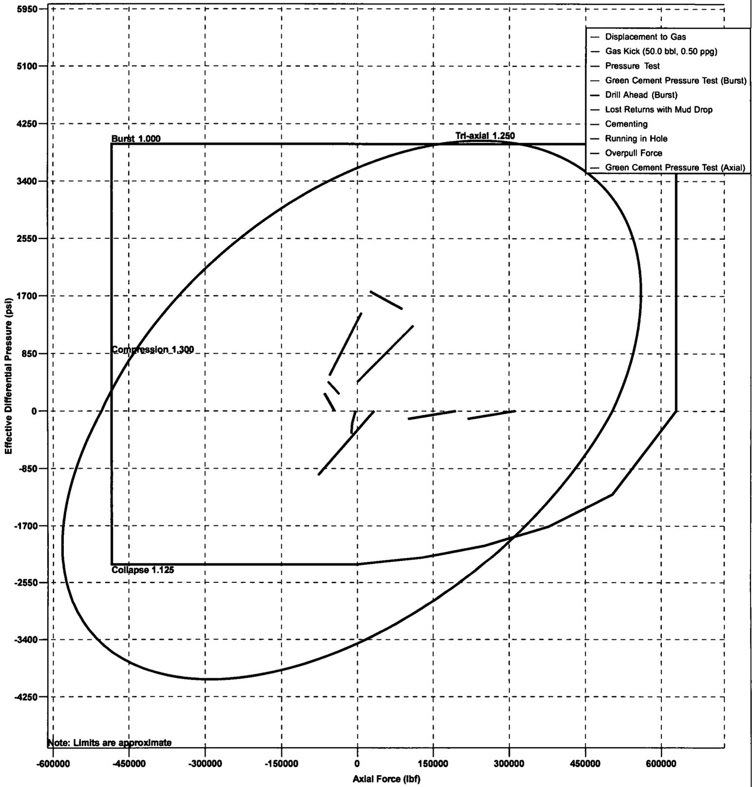
Design Limits (7" Production Casing - Section 1)
