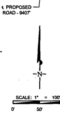
ALL BEARINGS, DISTANCES, AND COORDINATE VALUES CONTAINED HEREON ARE GRID BASED UPON THE NEW MEXICO STATE PLANE COORDINATE SYSTEM, EAST ZONE OF THE NORTH AMERICAN DATUM 1983, U.S. SURVEY FEET
