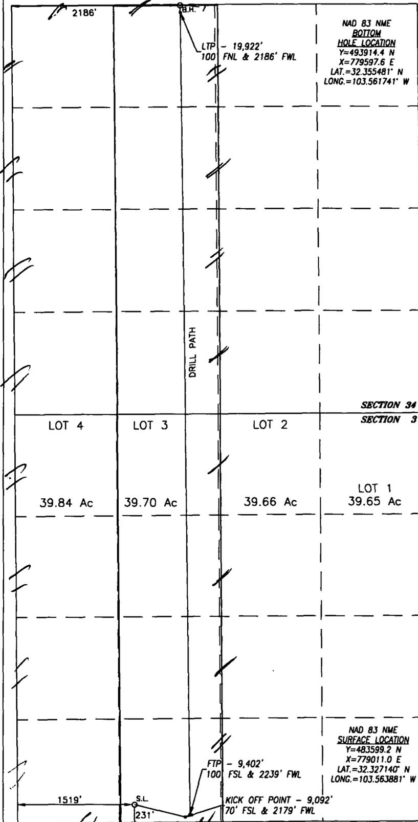
BOREPATH SHOWN HEREON IS BASED ON DIRECTIONAL SURVEY REPORT PROVIDED BY DEVON ENERGY PRODUCTION CO., L.P. FOR THE NORTH THISTLE 3-34 STATE COM #3H SUPPLIED TO HARCROW SURVEYING, LLC ON MAY 15, 2019
