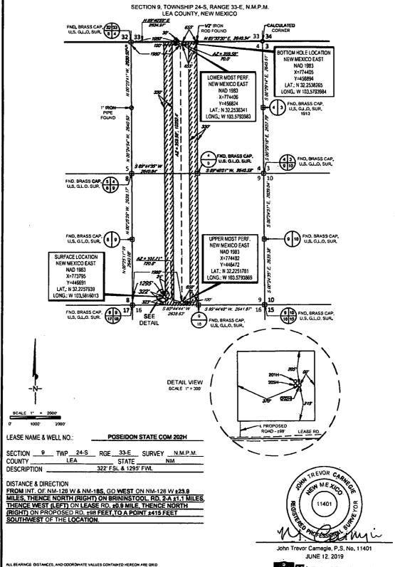
ALL BEARINGS. DISTANCES, AND COORDINATE VALUES CONTAINED HEREON ARE GRID BASED UPON THE NEW MEXICO COORDINATE SYSTEM OF 1983, EAST ZONE, U.S. SURVEY FEET.
