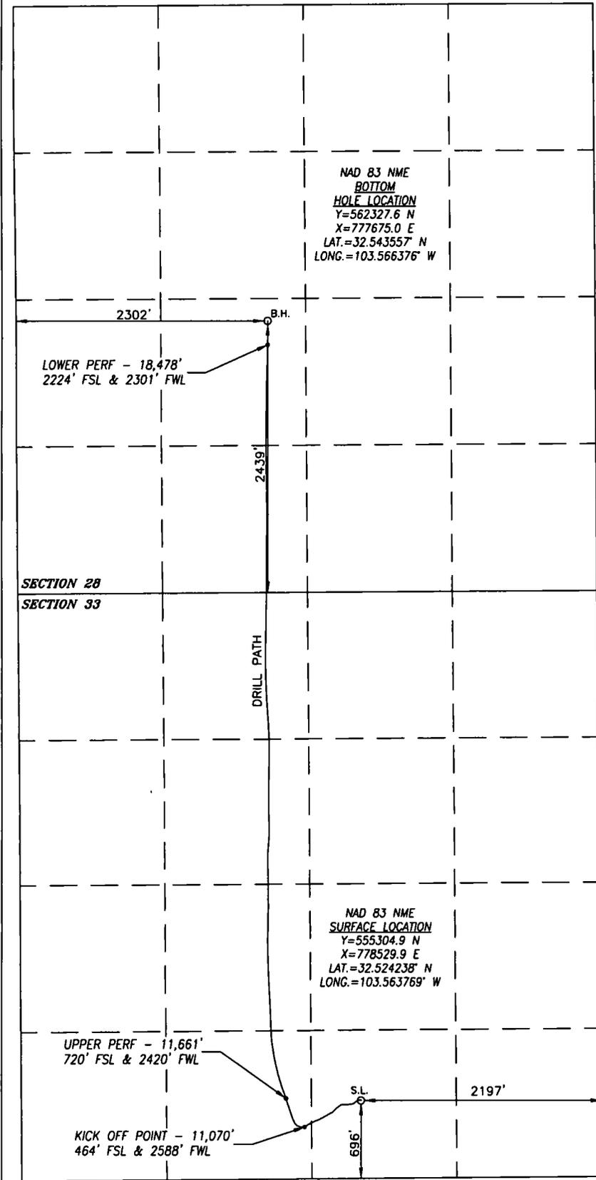
BOREPATH SHOWN HEREON IS BASED ON DIRECTIONAL SURVEY REPORT PROVIDED BY COG OPERATING, LLC FOR THE LITTLE BEAR FEDERAL COM #8H SUPPLIED TO HARCROW SURVEYING, LLC ON JULY 2, 2019
