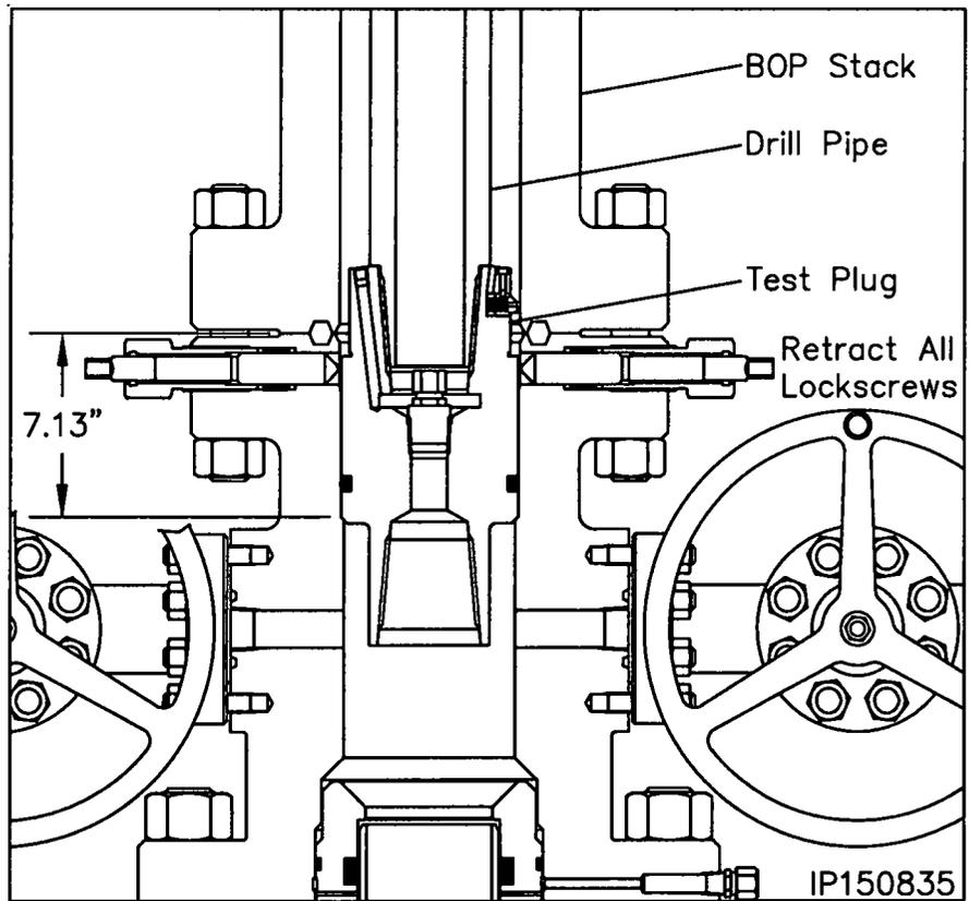
6. Carefully lower the test plug through the BOP and land it on the load shoulder in the tubing head, 7.13" below the top of the head.
