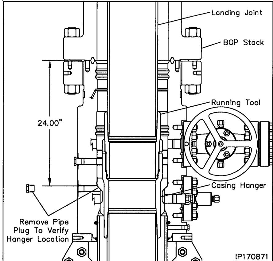
23. Reinstall the pipe plug and tighten securely.
