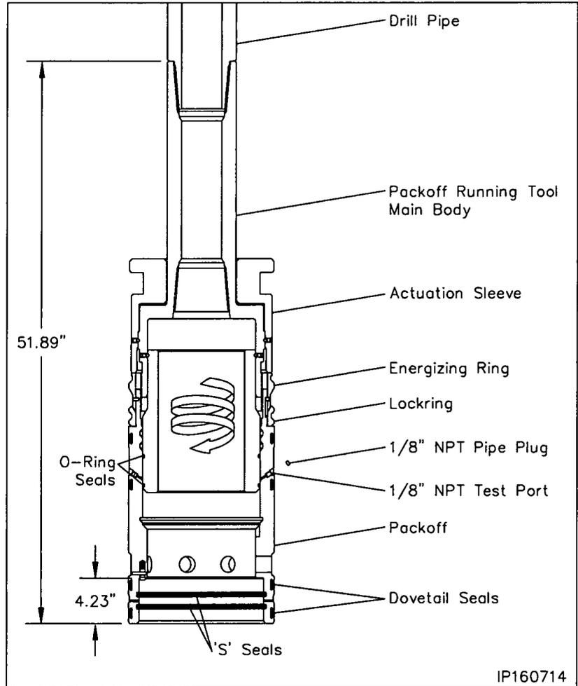
**WARNING:** All 1/8" pipe plugs must be removed prior to installing the packoff
