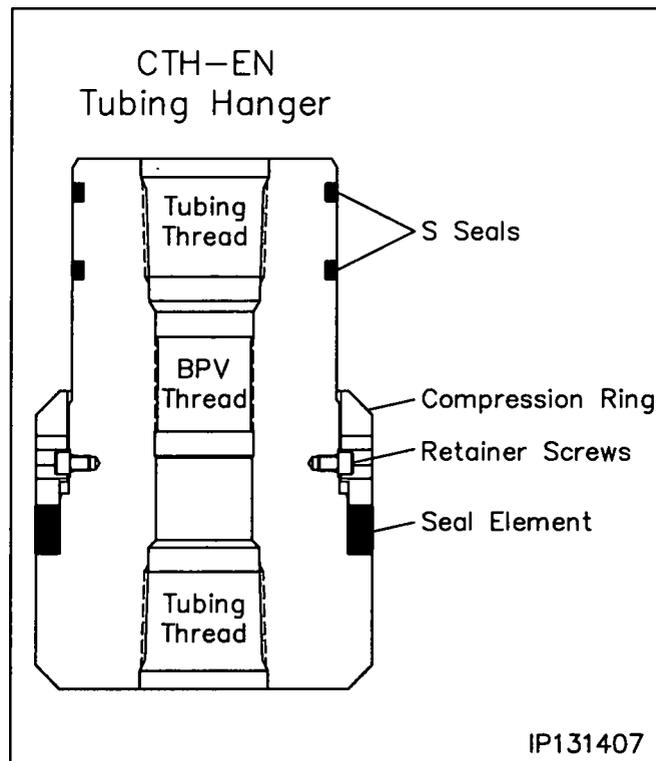
3. At a predetermined position in the tubing string, set the tubing in the floor slips. Pick up the Tubing Hanger and make it up in the tubing string. Torque the tubing hanger to the thread manufacturer's optimum make up torque.
