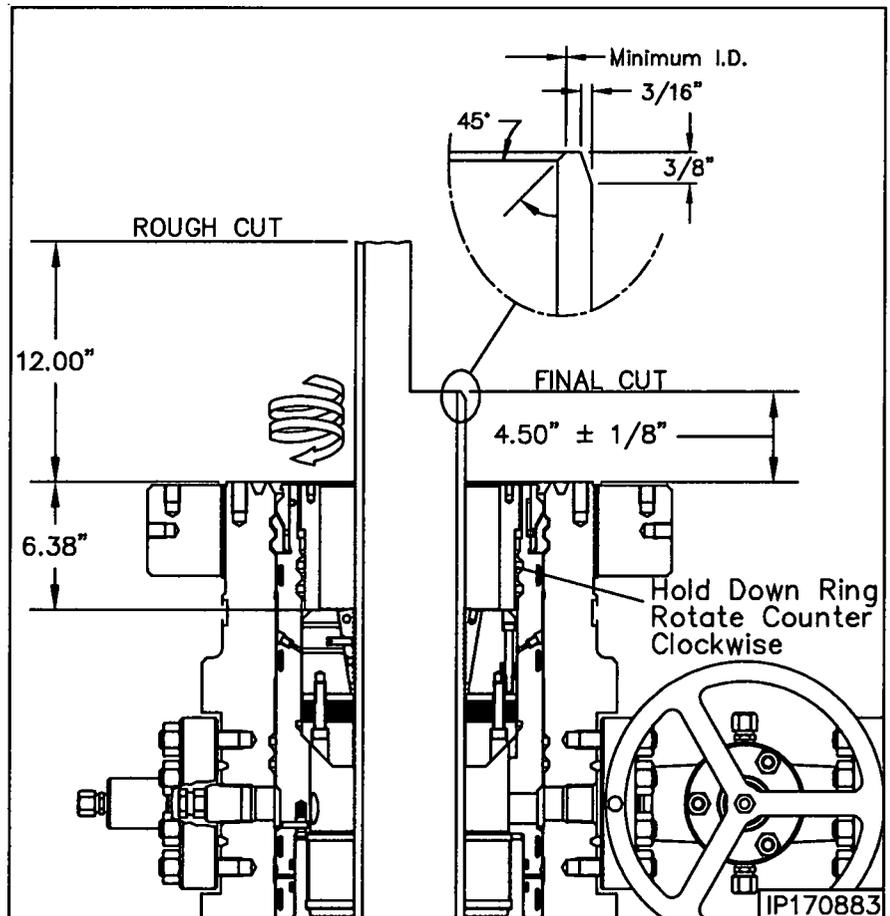
22. Using a high pressure water hose, thoroughly clean the top of the casing head, casing hanger, and casing stub and blow dry with compressed air. Ensure all cutting debris are removed.
