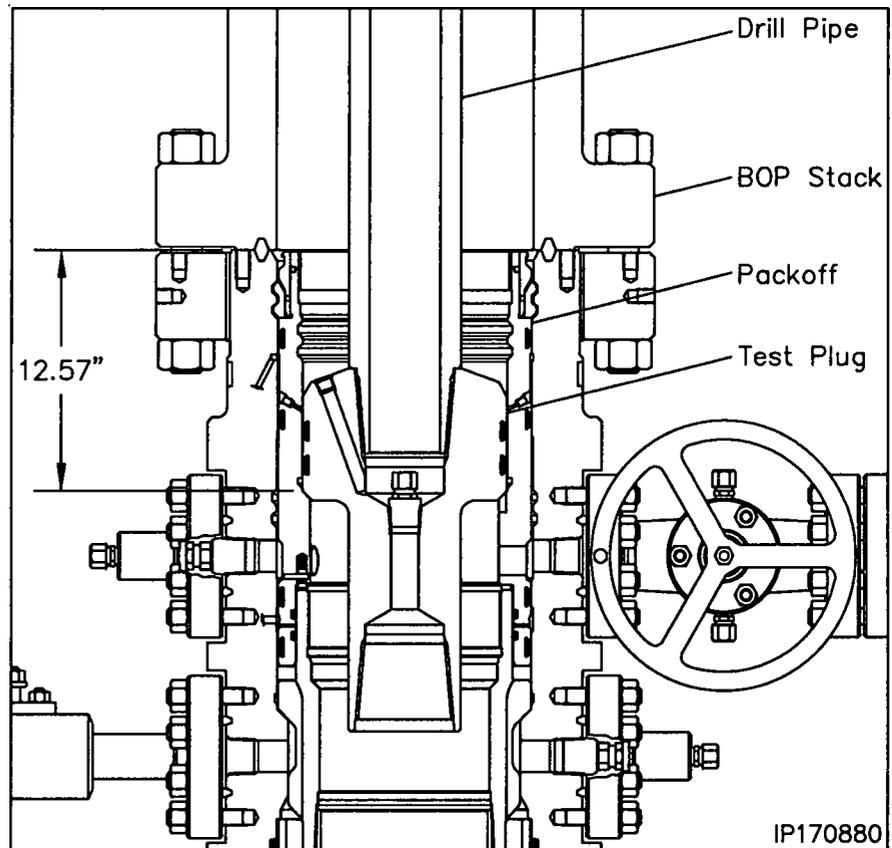
9. Remove as much fluid as possible from the BOP stack and retrieve the test plug with a straight vertical lift.
