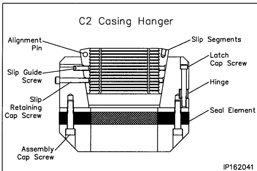
**Note:** Side outlet valve to remain open while setting the casing hanger.
