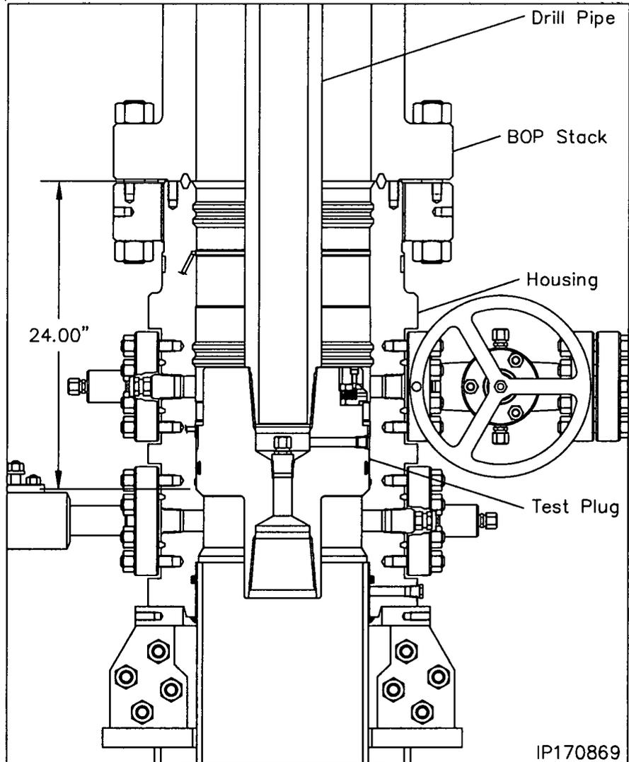
**Note:** When performing the BOP blind ram test it is highly recommended to suspend a stand of drill pipe below the test plug to ensure the plug stays in place while disconnecting it from the drill pipe.
