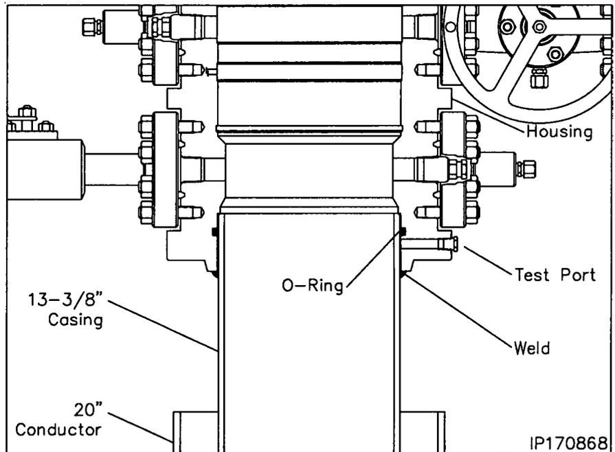
14. After a satisfactory test is achieved, replace the pipe plug in the port on the bottom of the housing.
