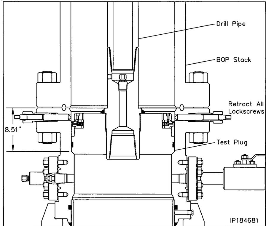
4. Open the casing head side outlet valve and fully retract all lockscrews.
