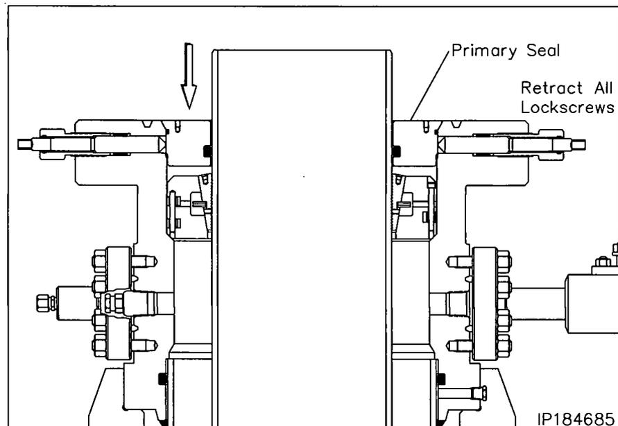
19. Carefully pass the plate over the casing stub and push it down until the mating 30° tappers of the plate and casing head make contact.
