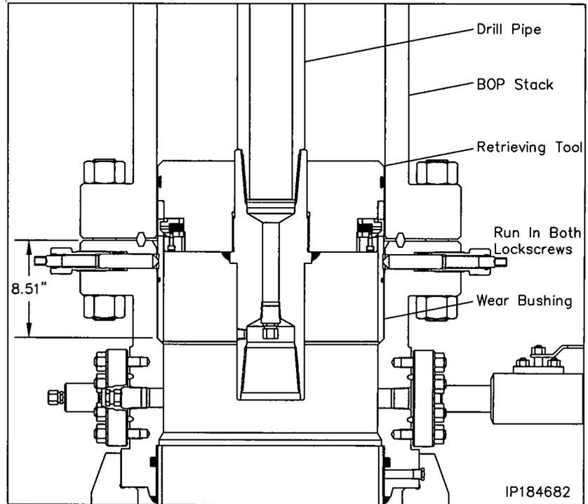
**Note:** It is highly recommended to retrieve, clean, inspect, grease, and reset the wear bushing each time the hole is tripped during the drilling of the hole section.
