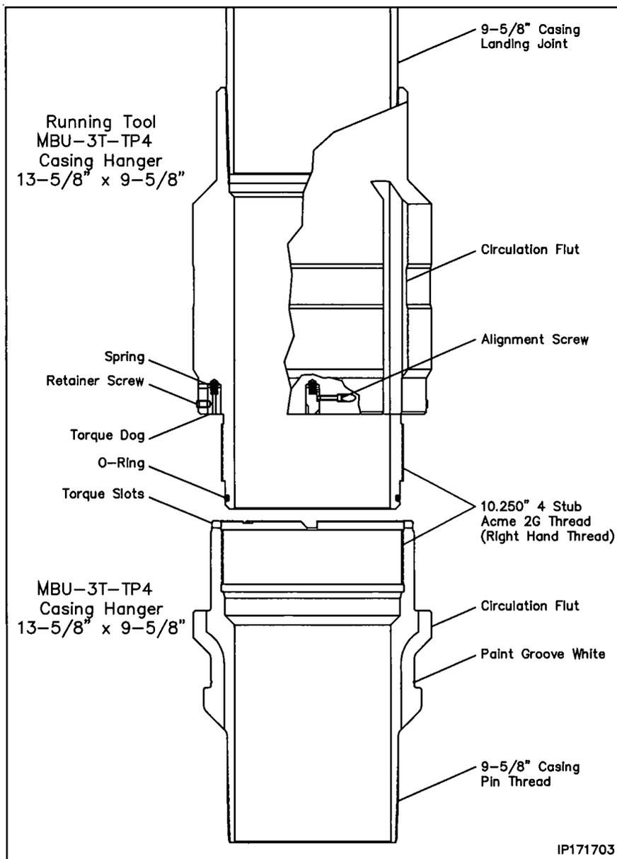
6. **Using chain tongs only**, thread the Running Tool into the hanger, with right hand rotation, until it shoulders out on the Hanger body.
