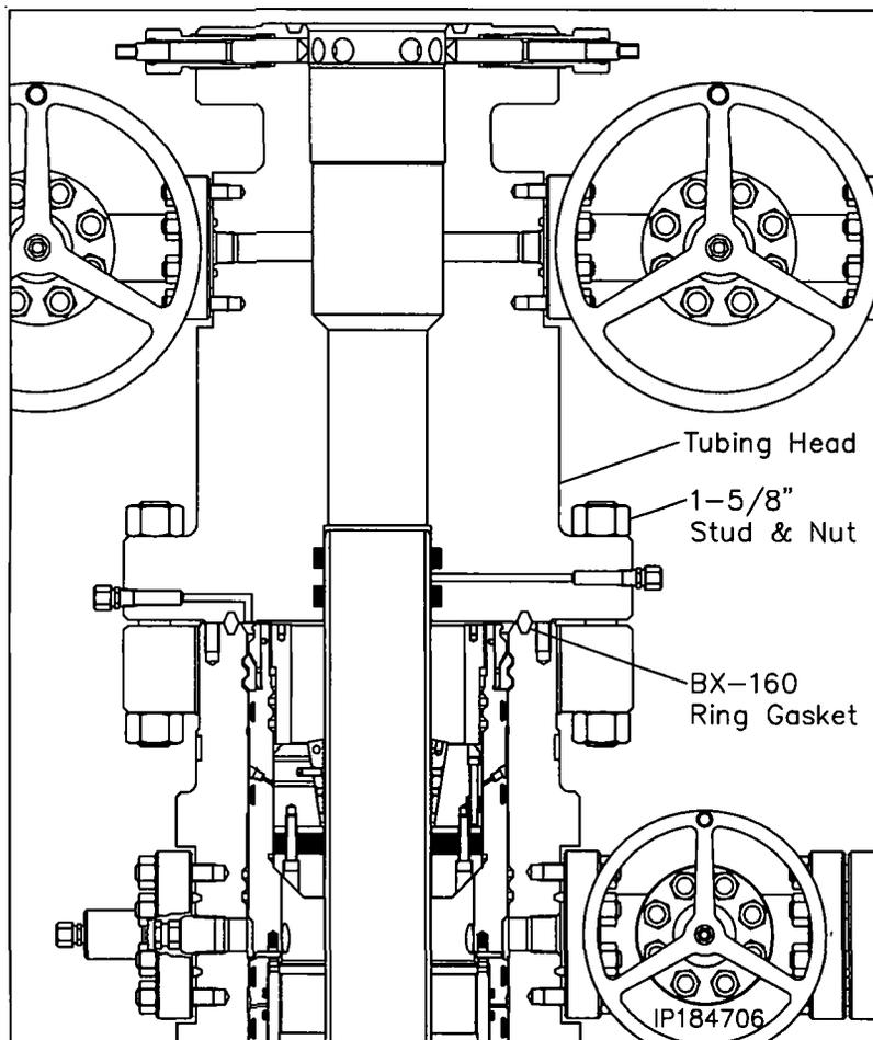
8. Lightly lubricate the I.D. of the tubing head 'HPS' seals and the casing stub with a light oil or grease.
