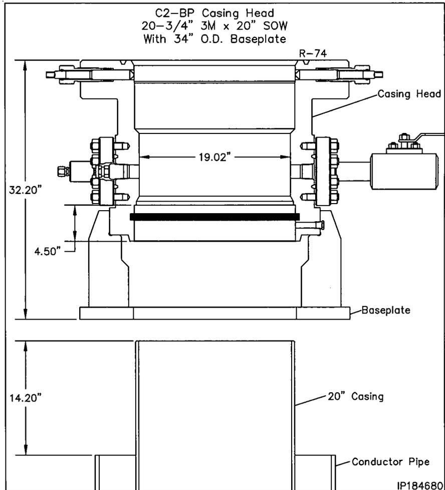
**Note:** The weld should be a fillet-type weld with legs no less than the wall thickness of the casing. Legs of 1/2" to 5/8" are adequate for most jobs.
