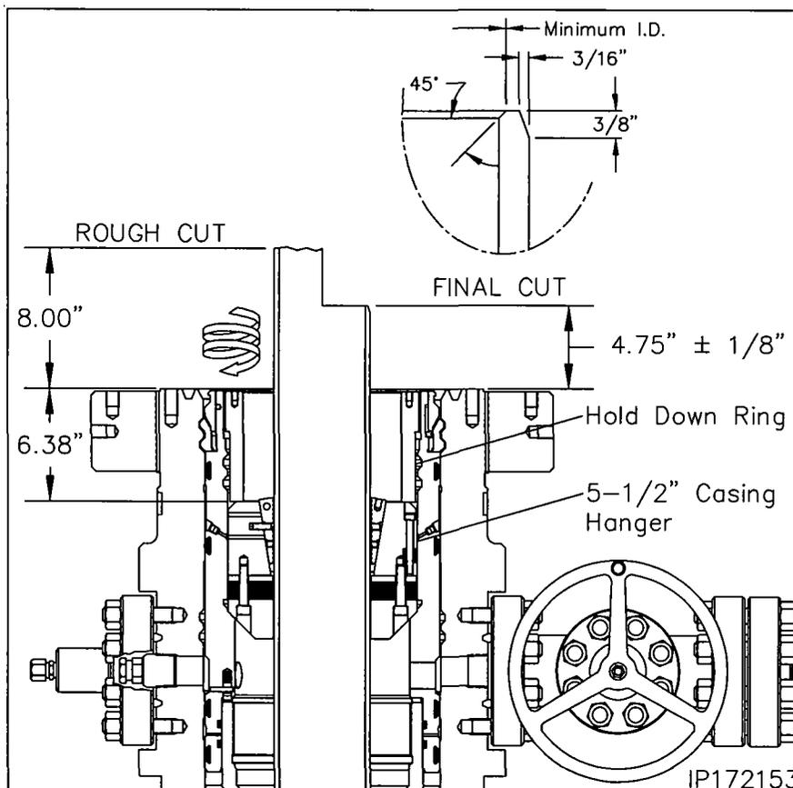
22. Using a high pressure water hose, thoroughly clean the top of the casing head, casing hanger, and casing stub and blow dry with compressed air. Ensure all cutting debris are removed.
