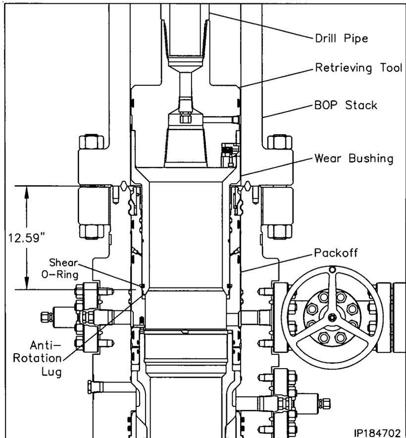
9. Remove the tool from the Wear Bushing by rotating the drill pipe counter clockwise (left) 1/4 turn and lifting straight up.
