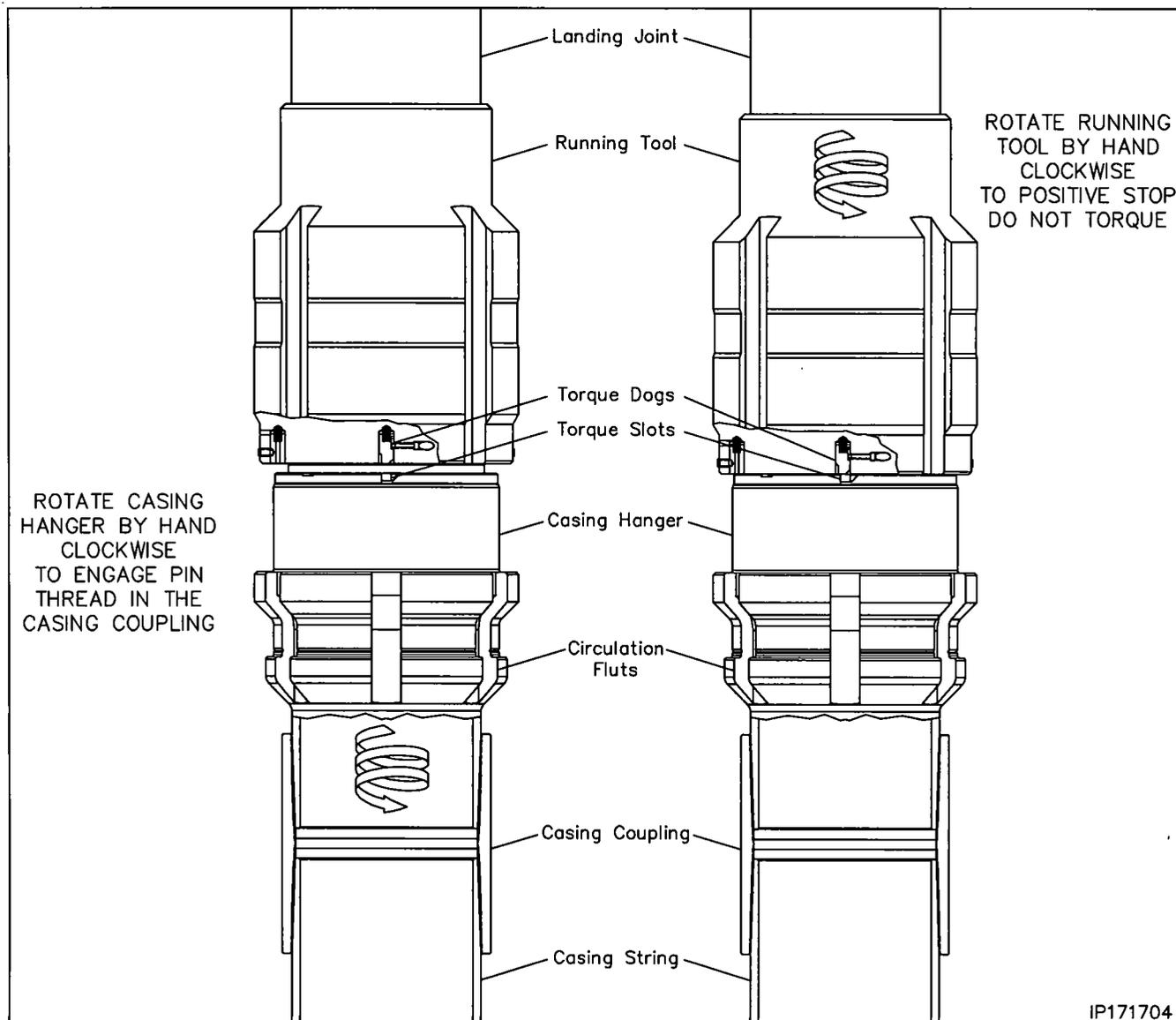
**Note:** If the 9-5/8" casing becomes stuck and the mandrel casing hanger cannot be landed, Refer to **Stage 9A** for the emergency procedure..
