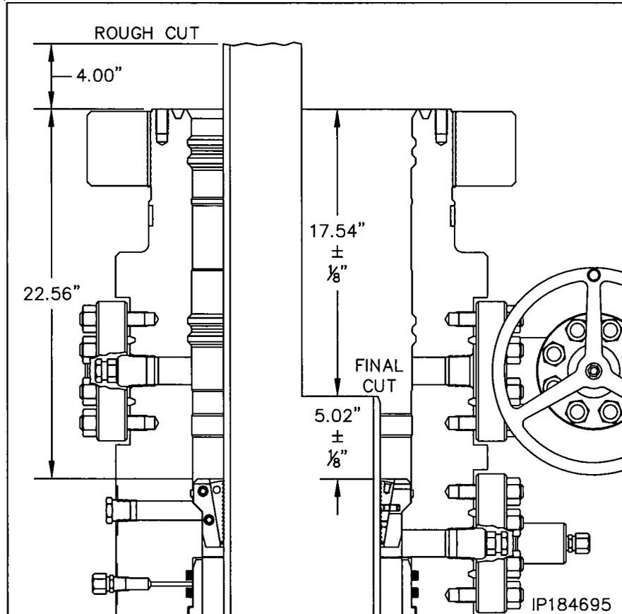
17. Rough cut the casing approximately 4" above the top of the housing and move the excess casing out of the way.
