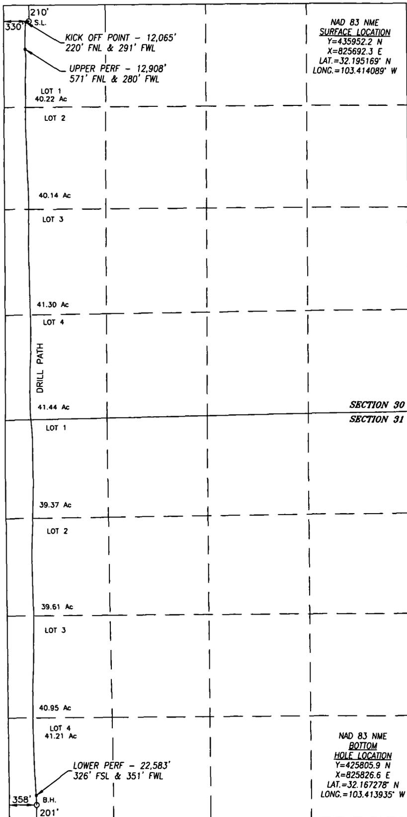
BOREPATH SHOWN HEREON IS BASED ON DIRECTIONAL SURVEY REPORT PROVIDED BY COG OPERATING, LLC FOR THE FASCINATOR FEDERAL COM #706H SUPPLIED TO HARCROW SURVEYING, LLC ON AUGUST 15, 2019
