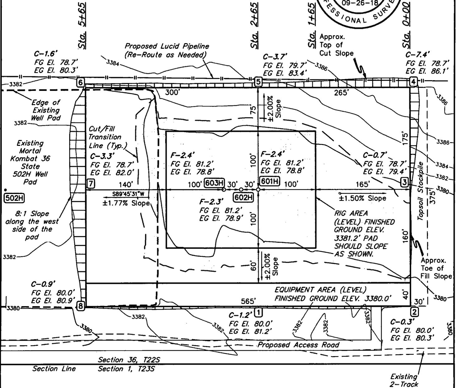
**NOTE:** Earthwork Calculations Require Fill @ the Location Stakes For Balance. All Fill is to be Compacted to a Minimum of 95% of the Maximum Dry Density Obtained by AASHTO Method t-99.
